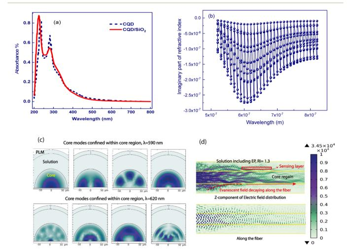
Fig. 5 (a) UV-Vis spectra of CQDs/MIPs, and (b) the calculated imaginary part of the refractive index as the function of the wavelength. (c and d) Mode profile of the norm of *E* and the corresponding *z* components of core-guided modes of CQDs/MIPs coated on optical fibers, from both views of the cross-section and along the optical fiber.
