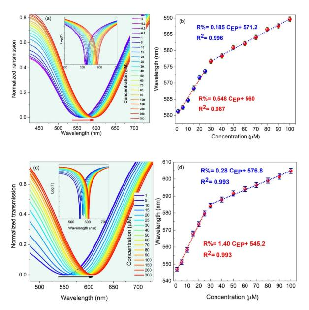
Effect of the elapsed time on the LMR shift, for (a and b) 3 h and (c and d) 7 h.
