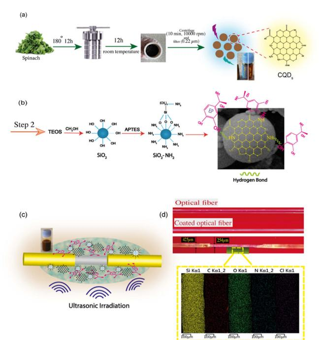
Fig. 1 (a) Schematic illustration of the synthesis of carbon dot nanoparticles from spinach; sample viewed under visible and ultraviolet light, (b) the chemical reaction at the core of the optical fiber, (c) immersed optical fiber in the solution under ultrasonic irradiation, (d) image of the surface-coated optical fiber along with the elemental mapping of the carbon dots.
