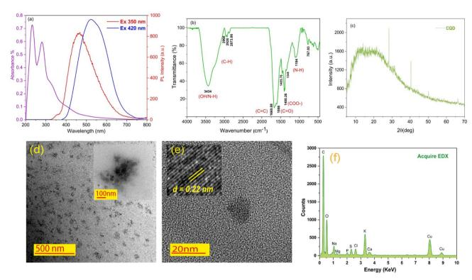
Fig. 2 (a) The UV-Vis absorption and PL intensity spectra at different excitation wavelengths of 350 and 420 nm, (b) FT-IR spectrum, (c) XRD pattern, (d) HR-TEM images, (e) magnified HR-TEM and inset showing the lattice fringe distance at 0.22 nm, and (f) EDX elemental mapping of the synthesized carbon dots.
