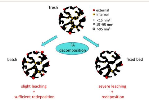
Fig. 8 Schematic of the leaching and redeposition behavior of the Pd@CMK3 catalyst during formic acid decomposition in the batch and the fixed bed reactors.
