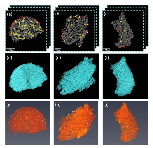
Fig. 6 Typical 2D slices from the reconstructed volume of Pd@CMK3 (a) before and after the FA decomposition reaction (b) in a batch reactor and (c) in a fixed bed reactor; the corresponding (d-f) surface renderings and (g-i) volume rendering. The red and yellow circles in (a)–(f) highlight Pd nanoparticles on the internal and external support surfaces.
