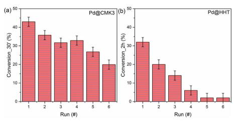
Fig. 3 Stability test during FA decomposition with a similar initial conversion: (a) Pd@CMK3 after 30 minutes of reaction time and (b) Pd@HHT after 2 hours of reaction time.
