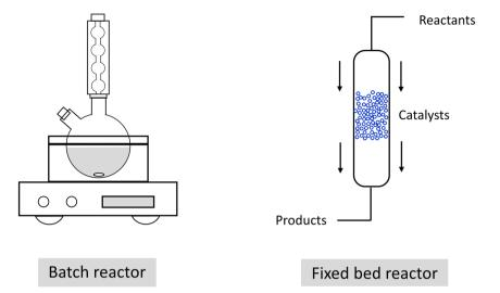
Fig. 1 Schematic diagram of a typical lab-used batch and fixed bed reactor.
