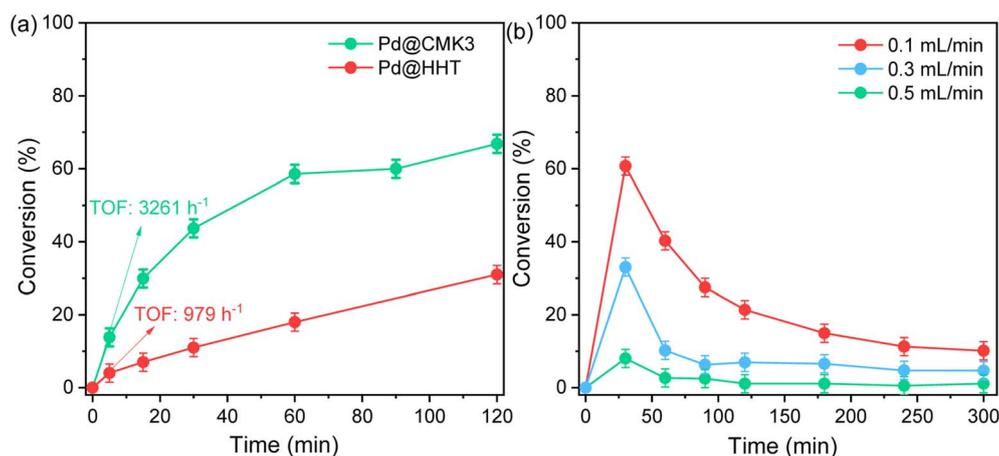
Fig. 2 Catalytic performance of Pd@CMK3 and Pd@HHT (from ref. 33) during FA decomposition. (a) FA conversion as a function of reaction time on Pd@CMK3 and Pd@HHT catalysts in the batch reactor. (b) FA conversion as a function of reaction time on Pd@CMK3 in the fixed bed reactor using flow rates of 0.1, 0.3 and 0.5 mL min<sup>-1</sup>.
