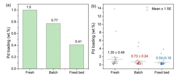
Fig. 5 Pd loading of Pd@CMK3 catalysts measured by (a) ICP-AES and (b) EDX based on around 30 regions of interest for each catalyst. SE in EDX data represents the standard error, which is defined as  $SE = std./\sqrt{n}$ , with std the standard deviation and n is the number of sample observations.
