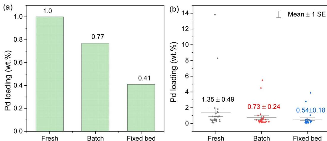
Fig. 5 Pd loading of Pd@CMK3 catalysts measured by (a) ICP-AES and (b) EDX based on around 30 regions of interest for each catalyst. SE in EDX data represents the standard error, which is defined as  $SE = \text{std.}/\sqrt{n}$ , with std the standard deviation and  $n$  is the number of sample observations.
