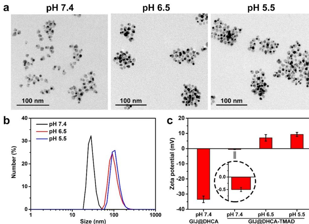
Fig. 2 *In vitro* acid-induced aggregation of GIJ@DHCA-TMAD. (a) The TEM images and (b) dynamic light scattering (DLS) of GIJ@DHCA-TMAD in 1× PBS buffer at different pH values (7.4, 6.5, and 5.5). (c) Zeta potential of GIJ@DHCA-TMAD and GIJ@DHCA.
