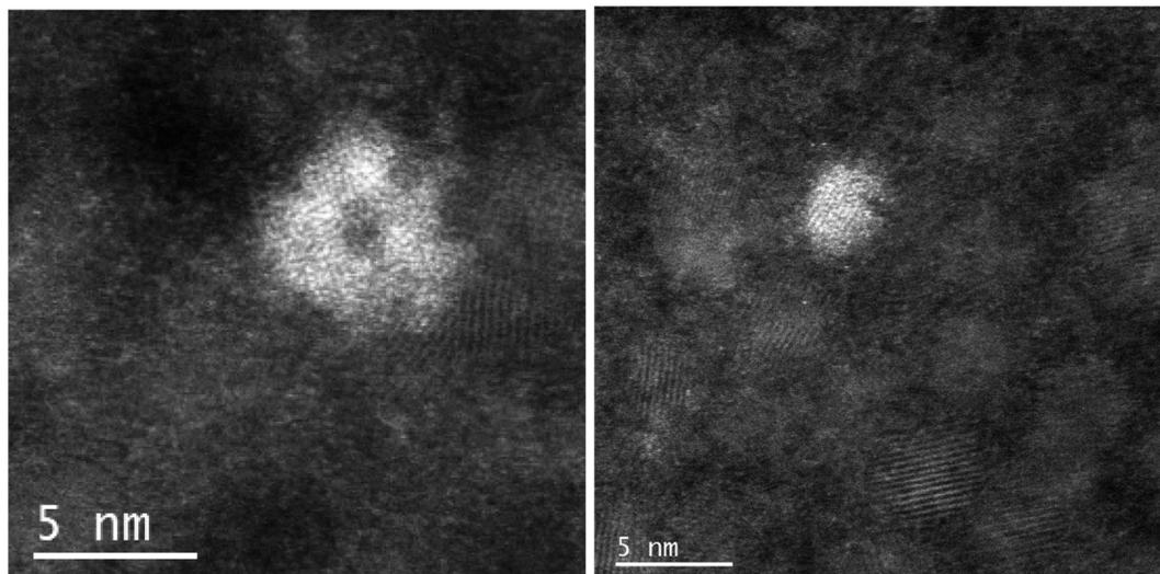
Fig. 3 Comparison of nascent iron cores of  $\sim 100$  Fe/protein loading for (A) L-rich and (B) H-rich heteropolymers. Site-directed iron nucleation produces distinctly different shapes of iron cores (see text for details).
