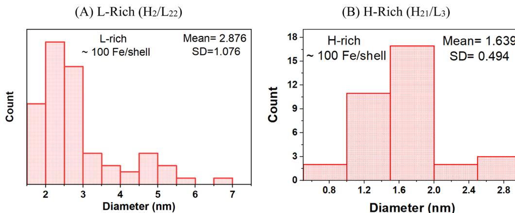
Fig. 4 Histograms of the particle size distributions of the ferrihydrite mineral cores grown in (A) L-rich heteropolymers and (B) H-rich heteropolymers, containing  $\sim 100$  Fe/protein.
