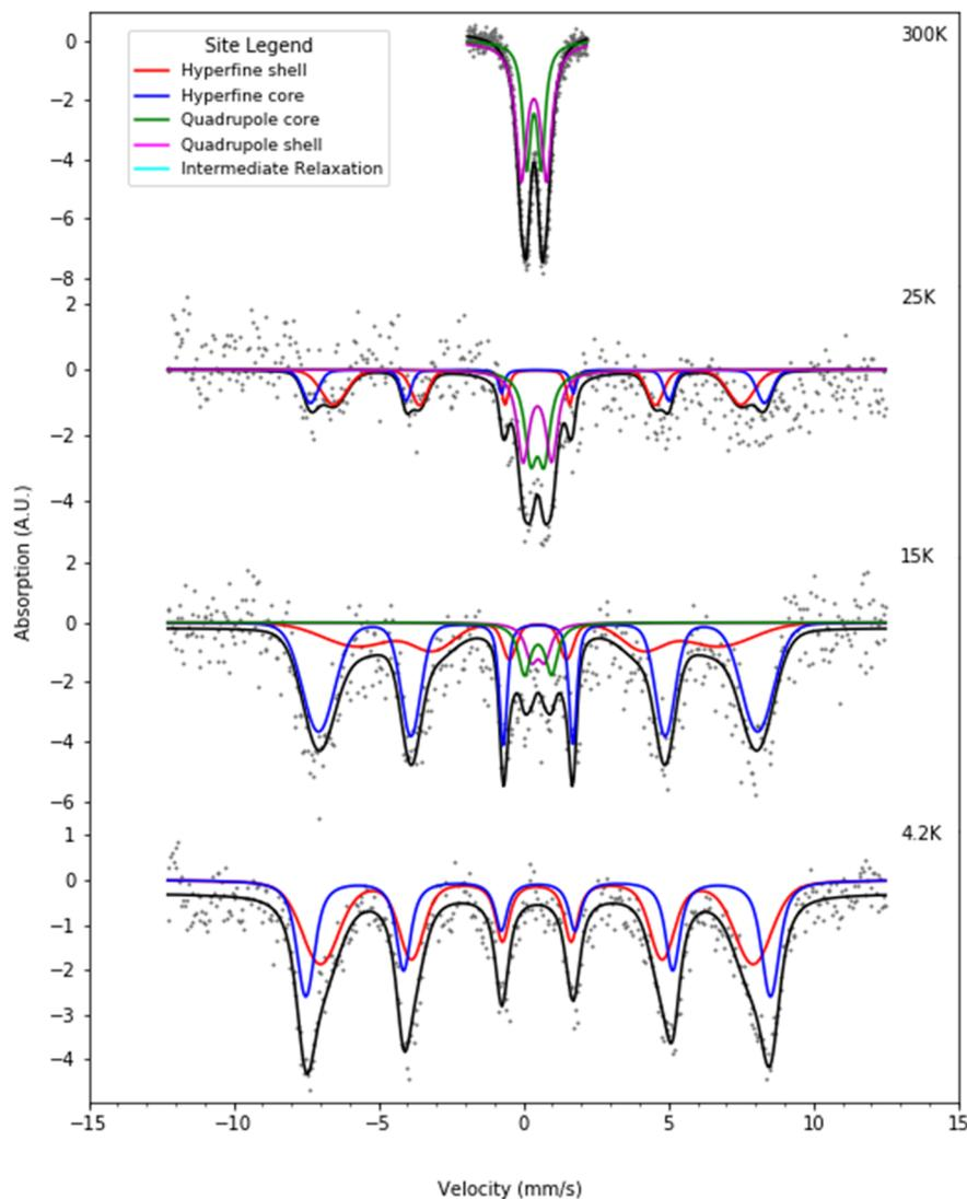
Fig. 6 Selected Mössbauer spectra for the L-rich heteropolymer ferritin reconstituted at 1000  $^{57}\text{Fe}$ /protein at various temperatures fitted to the core/shell model of the ferritin biomineral core (see site legend). Selected values of fitted parameters are given in Table 1.
