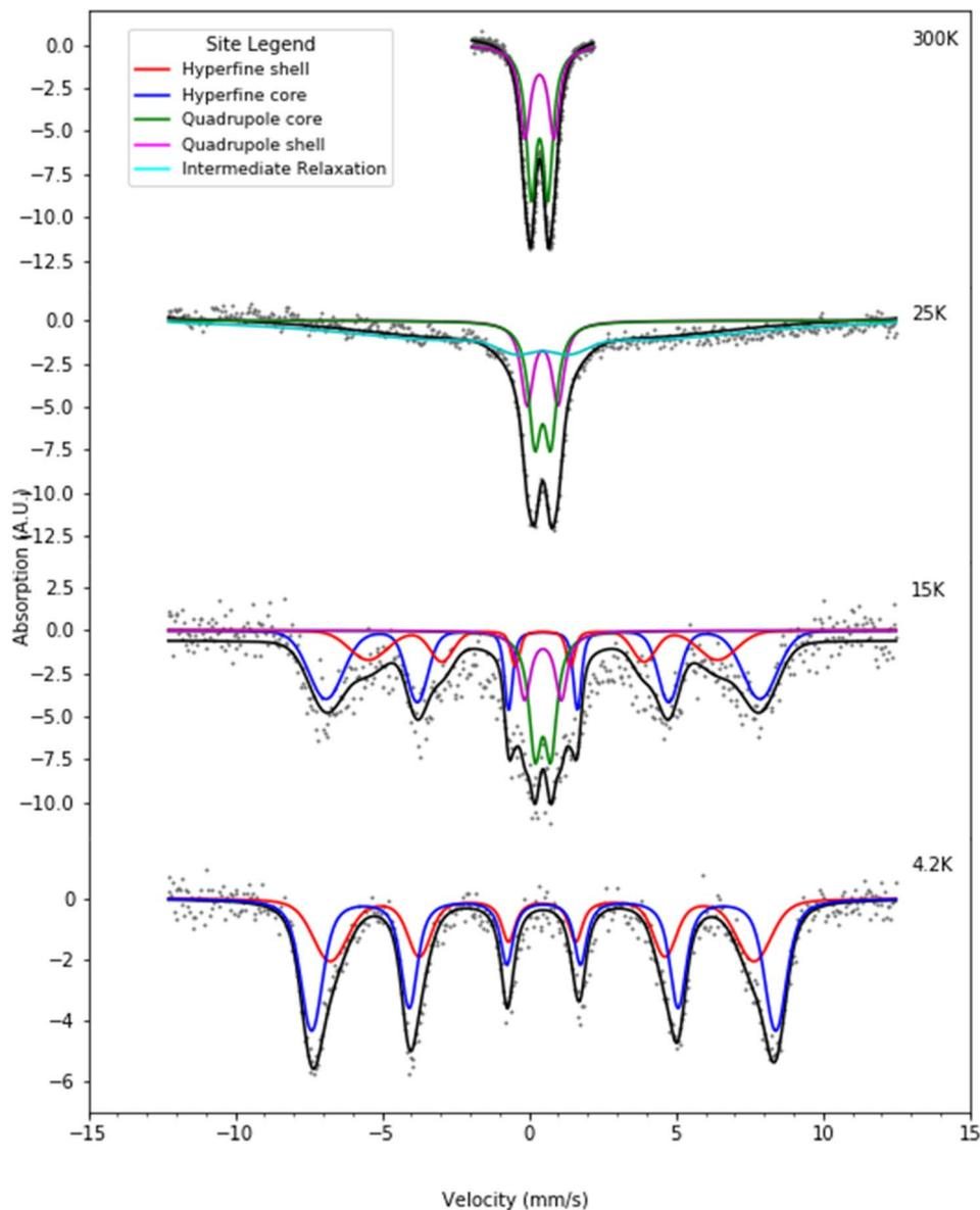
Fig. 7 Selected Mössbauer spectra for the H-rich heteropolymer ferritin reconstituted at 1000  $^{57}\text{Fe}$ /protein at various temperatures fitted to the core/shell model of the ferritin biomineral core (see site legend). Selected values of fitted parameters are given in Table 2.
