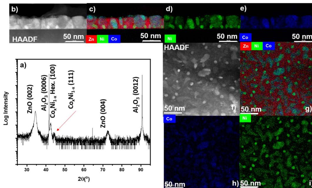
Fig. 3 Microstructural characterization of the ZnO– $\text{Co}_x\text{Ni}_{1-x}$  nanocomposite. (a)  $2\theta$  scan. (b) cross-section STEM. (c) Combined EDS-mapping. (d) EDS mapping Ni element. (e) EDS-mapping element. (f) In-plane STEM image. (g) Combined EDS-mapping plan-view. (h) EDS-mapping Co. (i) EDS-mapping Ni element.
