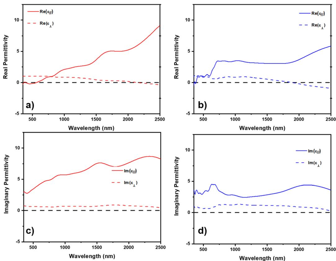
Fig. 5 Measured and model real and imaginary permittivity. Real permittivity for (a) ZnO–Ni and (b) ZnO–Co<sub>x</sub>Ni<sub>1-x</sub>. Imaginary permittivity for (c) ZnO–Ni and (d) ZnO–Co<sub>x</sub>Ni<sub>1-x</sub>.
