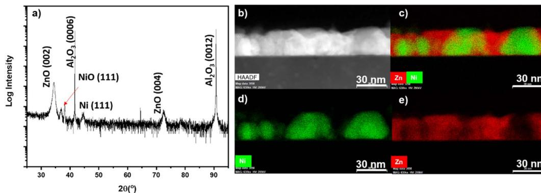
Fig. 2 Microstructural characterization of the ZnO–Ni nanocomposite. (a)  $2\theta$  scan. (b) Cross-section STEM image. (c) Combined EDS-mapping. (d) EDS-mapping for Ni. (e) EDS-mapping for Zn element.
