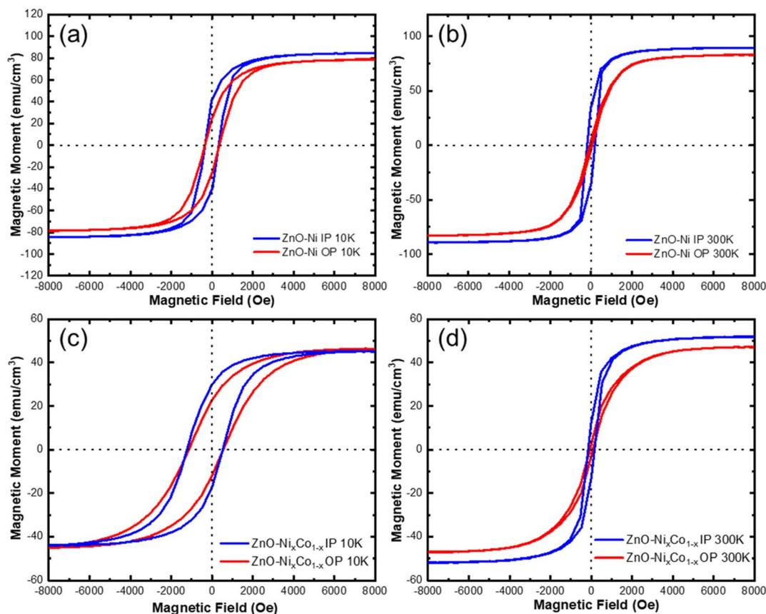
Fig. 4 Anisotropic magnetic measurement. (a) ZnO–Ni at 10 K, (b) ZnO–Ni at 300 K, (c) ZnO– $\text{Ni}_x\text{Co}_{1-x}$  at 10 K, (d) ZnO– $\text{Ni}_x\text{Co}_{1-x}$  at 300 K. Note that the diamagnetic responses from the non-magnetic holder and substrate were linearly subtracted from the original data using the slope calculated at high field (8000–10 000 Oe).
