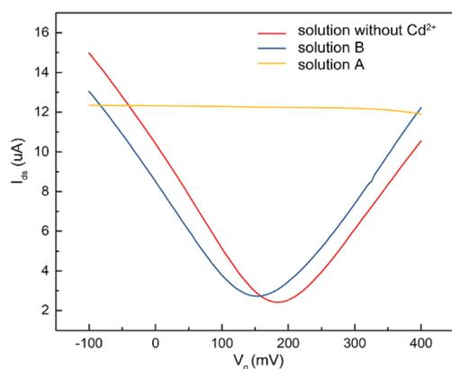
**Fig. 6** Transfer characteristic curves measured ( $V_{\text{ds}}$ : 10 mV) during exposure of the A-GFET detecting platform to oily wastewater with a  $\text{Cd}^{2+}$  concentration of 100 nM before (solution A) and after (solution B) filtration by the isolation membrane, respectively, showing that the isolation membrane could avoid the influence of oil on the test results effectively.
