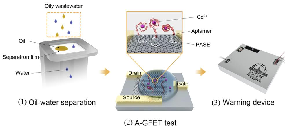
Fig. 1 Schematic diagram of the  $\text{Cd}^{2+}$ -detection process in oily wastewater. The detection can be divided into three processes: (1) oil–water separation, (2)  $\text{Cd}^{2+}$  detection using the A-GFET detecting platform, (3) analysis of the data and generation of an alarm signal by the PCB board.
