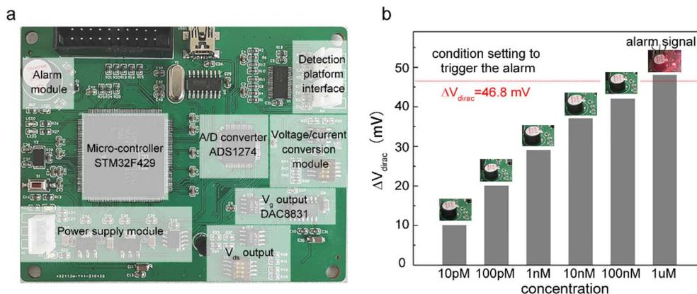
Fig. 4 (a) Circuit board used for collecting, analyzing, processing data, and sending an alarm signal. (b) The circuit part will send out a photo-acoustic alarm signal when the concentration of Cd<sup>2+</sup> in the tested solution rises to a certain concentration.
