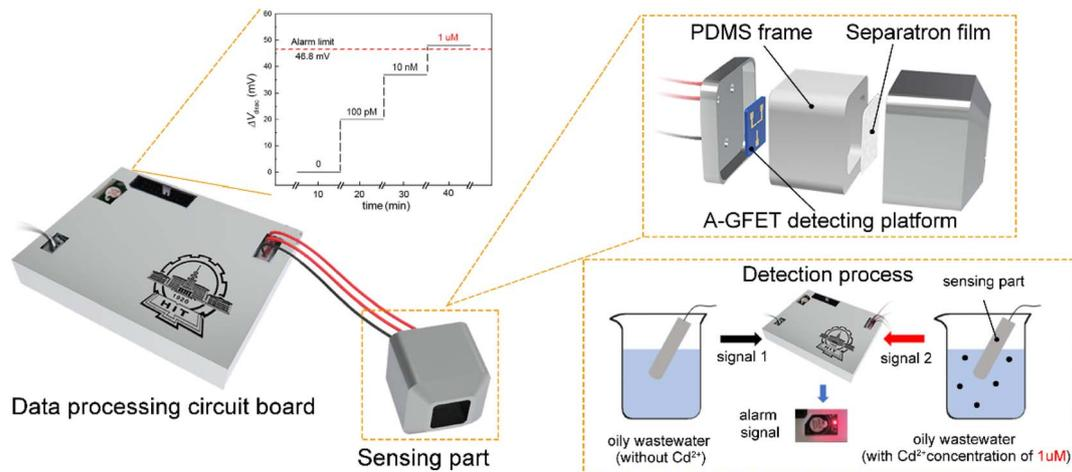
Fig. 7 Real-time monitoring and alarm system for  $\text{Cd}^{2+}$  in oily wastewater. The system will send out a photoacoustic alarm signal when the concentration of  $\text{Cd}^{2+}$  in the monitored liquid environment increases abnormally to exceed the safe value.
