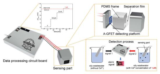
Fig. 7 Real-time monitoring and alarm system for  $Cd^{2+}$  in oily wastewater. The system will send out a photoacoustic alarm signal when the concentration of  $Cd^{2+}$  in the monitored liquid environment increases abnormally to exceed the safe value.
