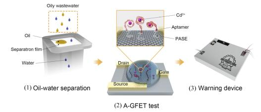
Fig. 1 Schematic diagram of the  $Cd^{2+}$ -detection process in oily wastewater. The detection can be divided into three processes: (1) oil-water separation, (2)  $Cd^{2+}$  detection using the A-GFET detecting platform, (3) analysis of the data and generation of an alarm signal by the PCB board.
