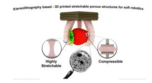
3D printing stretchable and compressible porous structures by polymerizable emulsions for soft robotics
