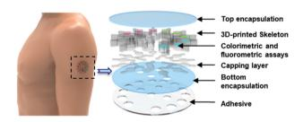
3D-printed epidermal sweat microfluidic systems with integrated microcuvettes for precise spectroscopic and fluorometric biochemical assays
