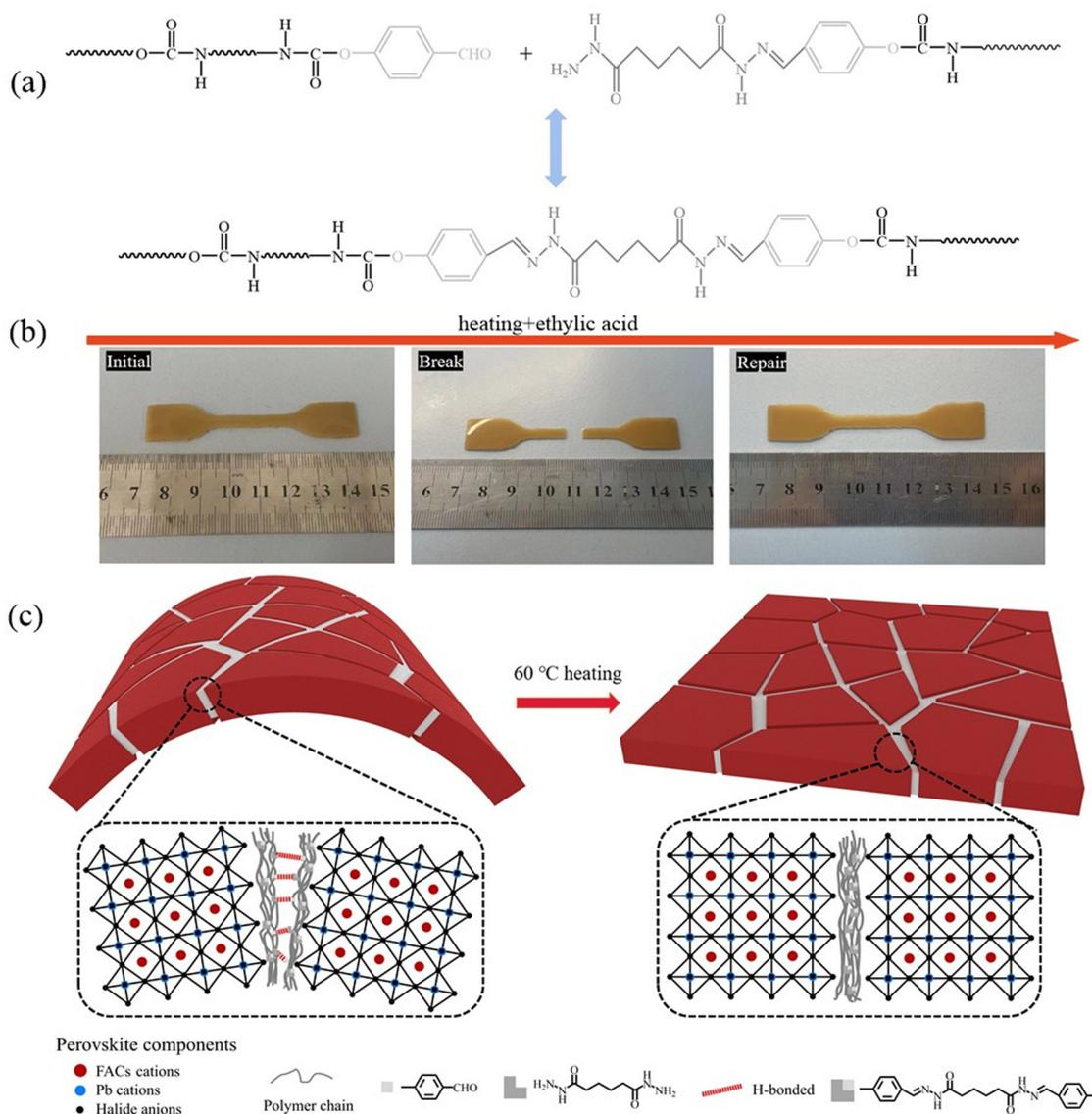
Fig. 6 (a) Schematic diagram of the Ab-WPU self-healing process, (b) Ab-WPU like self-healing experiment, and the (c) mechanism of Ab-WPU@perovskite membrane self-healing.
