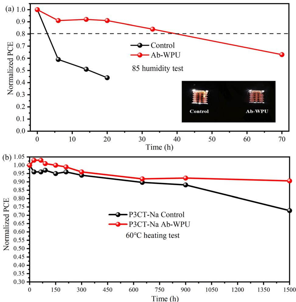
Fig. 7 (a) Normalized PCE plots of PSC devices without additives and modified with AB-WPU, stored in an 85% humidity environment (b) normalized PCE plots of PSC devices without additives and modified with AB-WPU, stored in an  $N_2$  environment at 60 °C.
