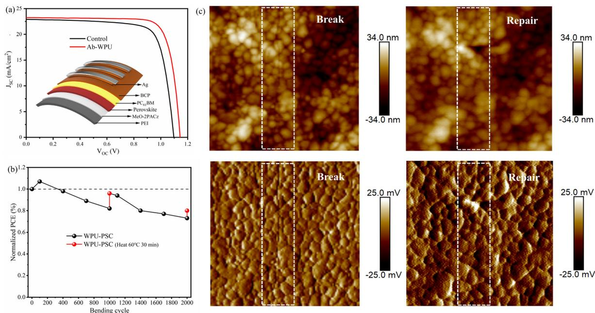
Fig. 5 (a) Structure diagram and  $J$ - $V$  curve of flexible perovskite solar cells without additives and modified with AB-WPU. (b) Bending resistance test of flexible perovskite solar cell devices treated with AB-WPU and efficiency test of device self-healing by heating at 1000 and 2000 bending cycles, respectively. (c) AFM images of cracks in perovskite films before and after self-healing (left and right).
