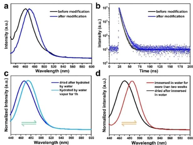
Fig. 5 Water stability of the modified CsPbBr<sub>3</sub>@W-S-1 composite. (a) Fluorescence spectra and (b) fluorescence lifetime decay of the CsPbBr<sub>3</sub>@W-S-1 composite and modified CsPbBr<sub>3</sub>@W-S-1 composite. Reversible PL properties of the modified CsPbBr<sub>3</sub>@W-S-1 composite (c) in water steam and (d) immersed in water.
