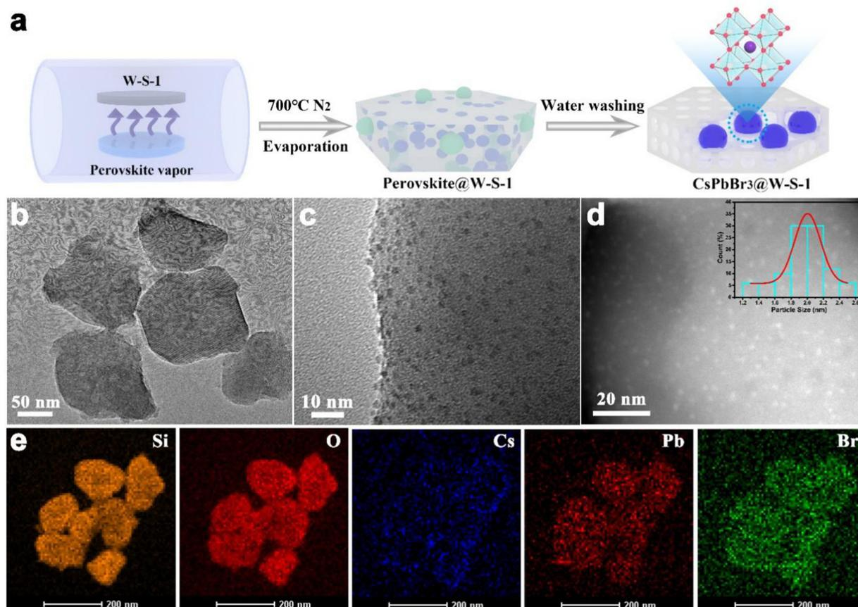
**Fig. 1** Synthetic procedure and morphology of the representative  $\text{CsPbBr}_3@W-S-1$  composite. (a) Schematic illustration of the synthetic procedure of the  $\text{CsPbBr}_3@W-S-1$  composite. (b) TEM and (c) HRTEM image of the  $\text{CsPbBr}_3@W-S-1$  composite. (d) STEM image of  $\text{CsPbBr}_3$  QDs distributed in a zeolite matrix. (e) EDX mapping images of Si, O, Cs, Pb and Br elements in the composite.
