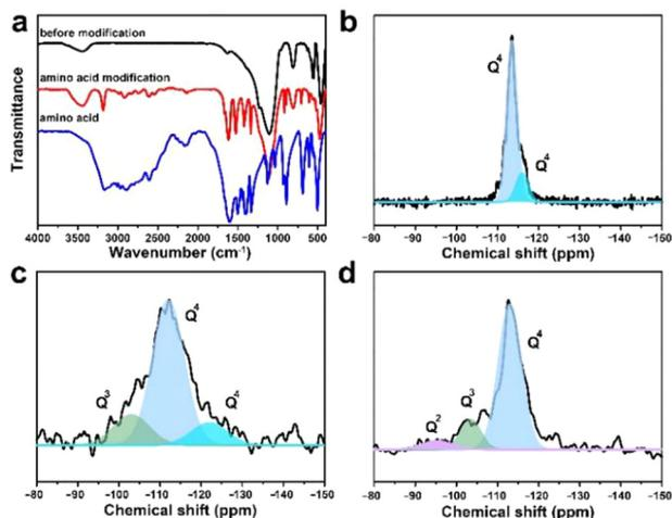
Fig. 4 Amino acid modification and silanization repaired CsPbBr<sub>3</sub>@W-S-1 composite. (a) FTIR spectra of the CsPbBr<sub>3</sub>@W-S-1 composite, modified CsPbBr<sub>3</sub>@W-S-1 composite and amino acid. <sup>29</sup>Si MAS NMR spectra of (b) W-S-1, (c) the CsPbBr<sub>3</sub>@W-S-1 composite and (d) the modified CsPbBr<sub>3</sub>@W-S-1 composite.
