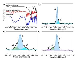
Fig. 4 Amino acid modification and silanization repaired CsPbBr $_3$ @W-S-1 composite. (a) FTIR spectra of the CsPbBr $_3$ @W-S-1 composite, modified CsPbBr $_3$ @W-S-1 composite and amino acid. <sup>29</sup>Si MAS NMR spectra of (b) W-S-1, (c) the CsPbBr $_3$ @W-S-1 composite and (d) the modified CsPbBr $_3$ @W-S-1 composite.
