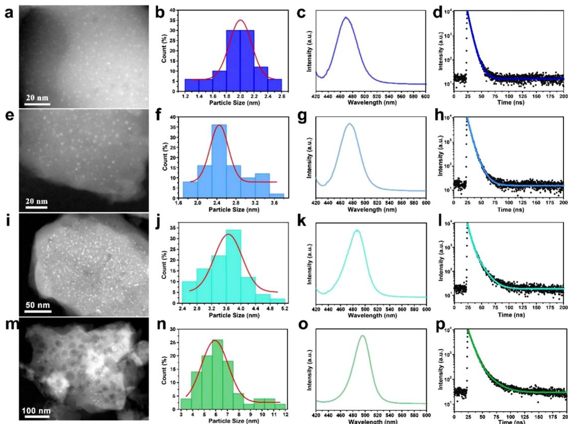
Fig. 2 Morphology and optical properties of CsPbBr<sub>3</sub>@W-S-1 composites obtained in different conditions. (a), (e), (i) and (m) STEM images of various sized CsPbBr<sub>3</sub> PQDs confined in the W-S-1 matrix and (b), (f), (j) and (n) the corresponding size distribution. (c), (g), (k) and (o) Fluorescence spectra of the corresponding CsPbBr<sub>3</sub>@W-S-1 composites, and (d), (h), (l) and (p) their fluorescence lifetime decay spectra, excited by 400 nm light.
