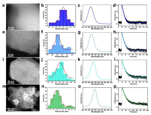
Fig. 2 Morphology and optical properties of  $CsPbBr_3@W-S-1$  composites obtained in different conditions. (a), (e), (i) and (m) STEM images of various sized  $CsPbBr_3$  PQDs confined in the W-S-1 matrix and (b), (f), (j) and (n) the corresponding size distribution. (c), (g), (k) and (o) Fluorescence spectra of the corresponding  $CsPbBr_3@W-S-1$  composites, and (d), (h), (l) and (p) their fluorescence lifetime decay spectra, excited by 400 nm light.
