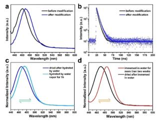
Fig. 5 Water stability of the modified CsPbBr<sub>3</sub>@W-S-1 composite. (a) Fluorescence spectra and (b) fluorescence lifetime decay of the CsPbBr<sub>3</sub>@W-S-1 composite and modified CsPbBr<sub>3</sub>@W-S-1 composite. Reversible PL properties of the modified CsPbBr<sub>3</sub>@W-S-1 composite (c) in water steam and (d) immersed in water.
