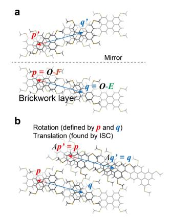
Fig. 4 Construction of the neighboring layer in the iBW structure of MTperylene from the BW structure. The mirror plane can be chosen arbitrarily and is y = 8.5 Å in the present case (a). Rotation matrix A in (b) is defined in eqn (1) to ensure  $A\mathbf{q}' = \mathbf{q}$  (and  $A\mathbf{p}' = \mathbf{p}$ ).
