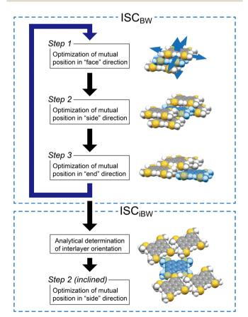
Fig. 5 Schematic representation of the ISC protocol for BW structures (ISC<sub>BW</sub>) and renewed ISC covering iBW structures (ISC<sub>iBW</sub>).
