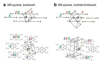
Fig. 6 Crystal structures of MS-pyrene featuring BW (a) and iBW (b) structures. The structures are shown from the side (top) and top (bottom) of the molecular plane.
