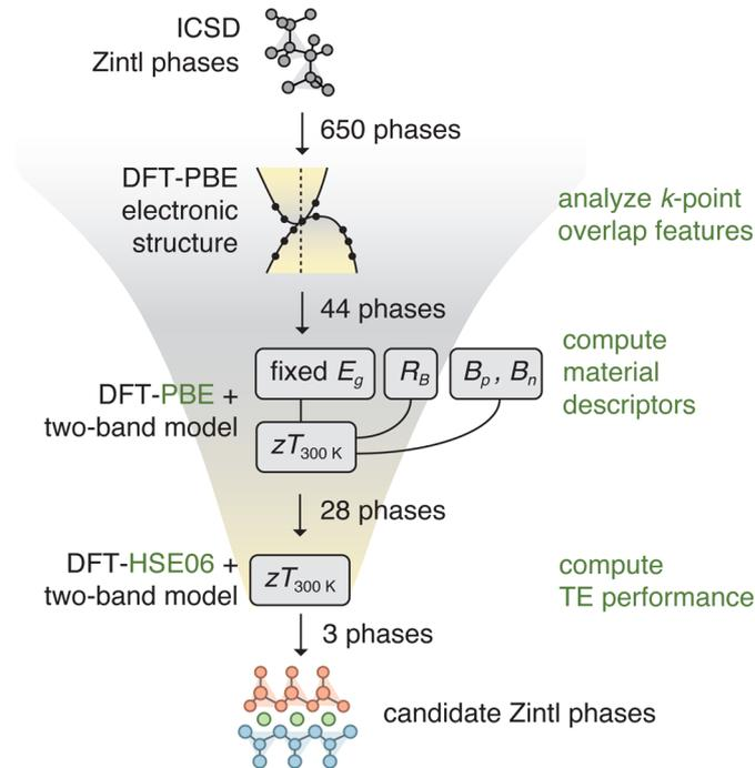
Fig. 4 Computational workflow to identify Zintl phases that are narrow-gap semiconductors or semimetals and exhibit high room-temperature thermoelectric performance.  $E_g$  is the band gap,  $R_B$  is the asymmetry parameter, and  $B_{\text{maj}}$  and  $B_{\text{min}}$  are the quality factors of majority and minority carriers. PBE and HSE06 refer to DFT functionals (see Methods).
