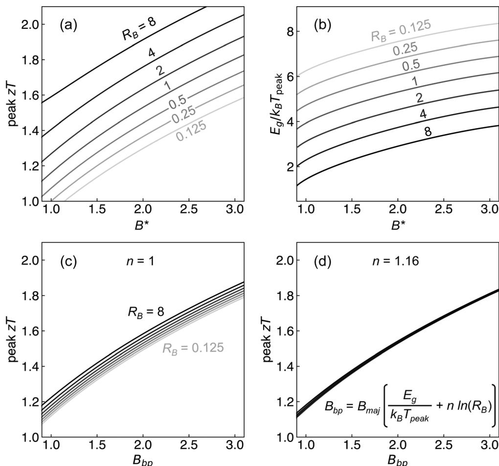
Fig. 6 (a) Peak  $zT$  and (b)  $E_g/k_B T_{\text{peak}}$  plotted against  $B^*$  (eqn (17)) for different values of  $R_B$ . Peak  $zT$  plotted against  $B_{\text{bp}}$  (eqn (18)) is shown for (c)  $n = 1$  and (d)  $n = 1.16$ .
