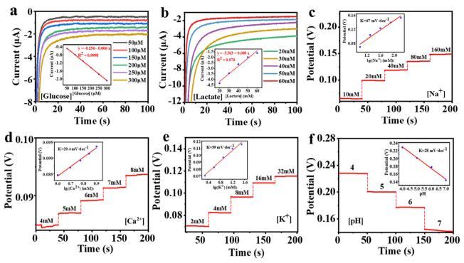
Fig. 4 The sensing performance of the electrochemical sensing fibers. The chronoamperometric responses of the glucose (a) and lactate (b) sensors to the respective analyte solutions in phosphate-buffered saline (PBS). (c)-(f) Open-circuit potential responses of the electrochemical sensing fibers to Na<sup>+</sup>, Ca<sup>2+</sup>, K<sup>+</sup>, and pH in respective analyte solutions, respectively.
