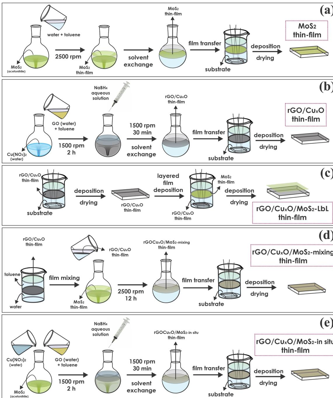
Fig. 1 Schematic representation of the general steps for the thin film preparation: (a) MoS<sub>2</sub>; (b) rGO/Cu<sub>x</sub>O or rGO; (c) rGO/MoS<sub>2</sub>-LbL and rGO/Cu<sub>x</sub>O/MoS<sub>2</sub>-LbL; (d) rGO/MoS<sub>2</sub>-mixing and rGO/Cu<sub>x</sub>O/MoS<sub>2</sub>-mixing; (e) rGO/MoS<sub>2</sub>-in situ and rGO/Cu<sub>x</sub>O/MoS<sub>2</sub>-in situ.
