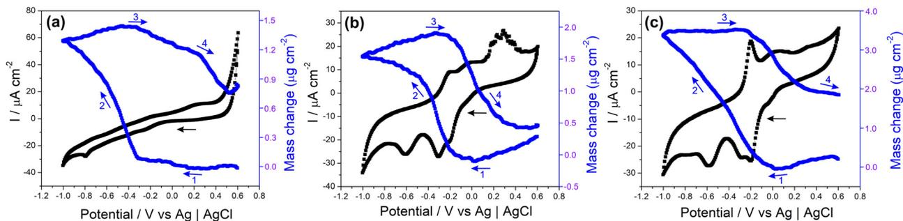
Fig. 7 Cyclic voltammograms (black) and evolution of the film mass (blue) during the third cycle (arrows indicate the scanning direction) for the MoS<sub>2</sub> (a), rGO/Cu<sub>x</sub>O (b) and rGO/Cu<sub>x</sub>O/MoS<sub>2</sub>-*in situ* (c) films. Conditions: Gold/quartz substrate, NaCl electrolyte (0.1 mol L<sup>-1</sup>) and scan rate 10 mV s<sup>-1</sup>.
