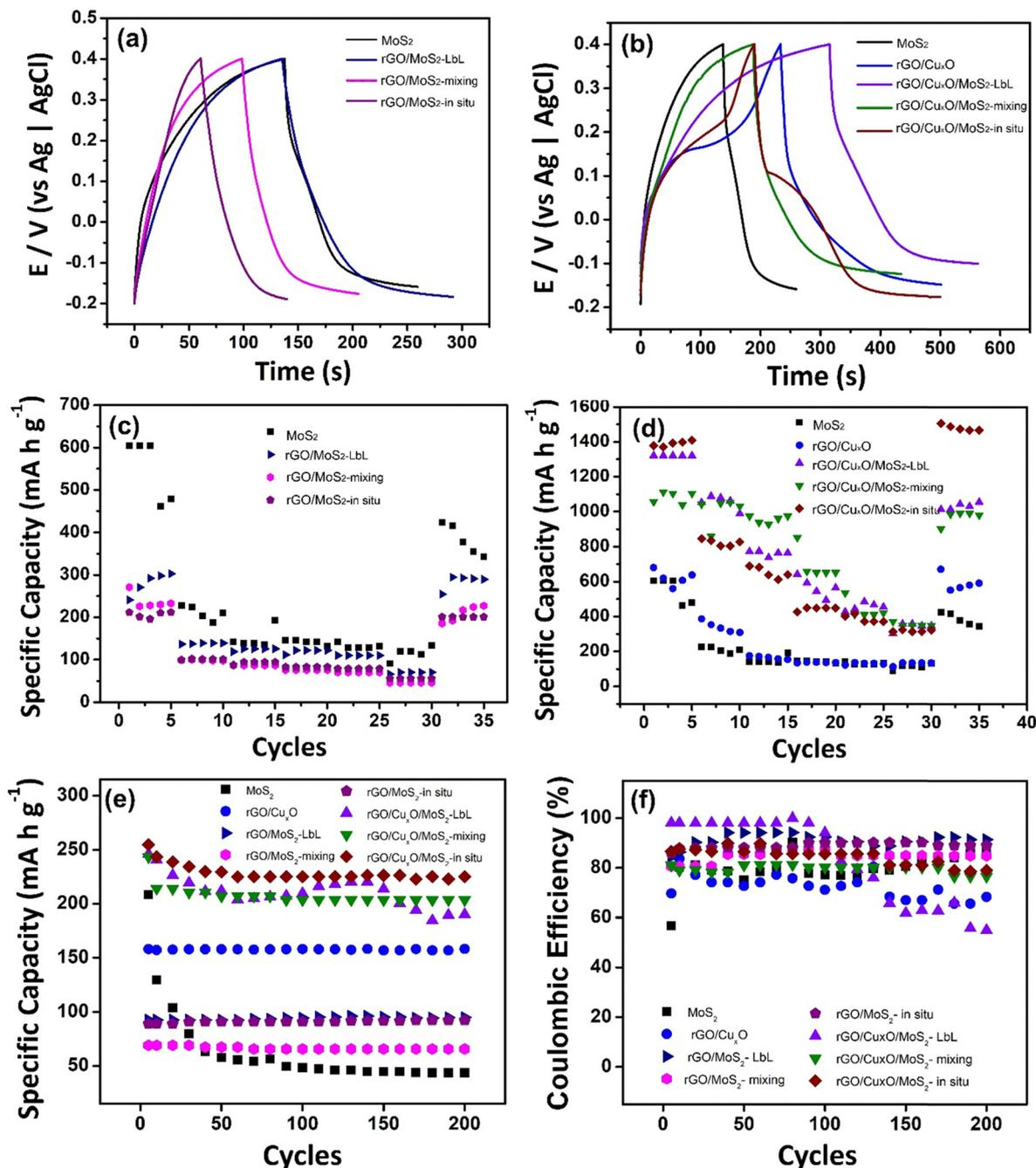
Fig. 8 Charge and discharge curves (a) and (b); specific capacity of the discharge process (c) and (d) at different current densities (0.1, 0.25, 0.5, 0.75, 1 and 2 A g<sup>-1</sup>); specific capacity measured during 200 cycles at 2 A g<sup>-1</sup> (e) and Coulombic efficiency (f) of the nanocomposites in 0.1 mol L<sup>-1</sup> NaCl aqueous solution and the potential range of -0.2 to 0.4 V.
