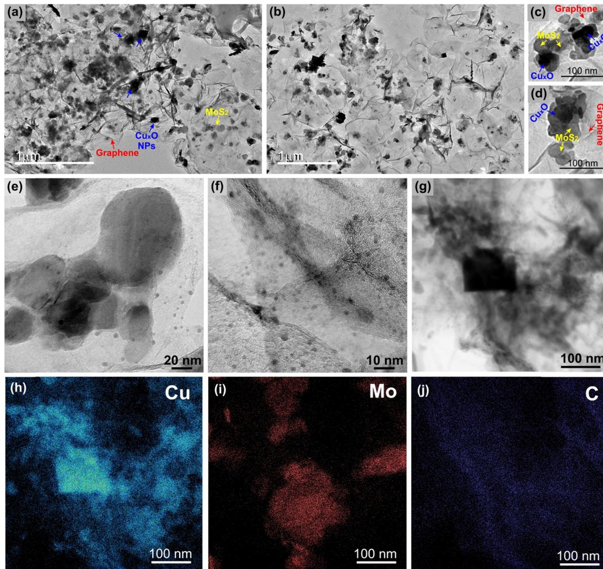
Fig. 5 Transmission electron microscopy images (a)–(g) and energy dispersive spectroscopy mapping images (h)–(j) of the rGO/Cu<sub>x</sub>O/MoS<sub>2</sub>-*in situ* sample.
