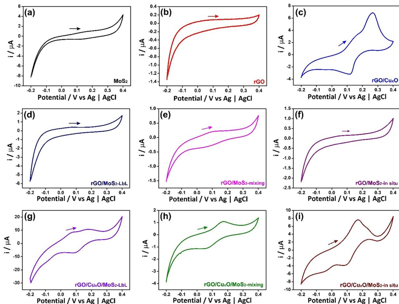
Fig. 6 Cyclic voltammograms of the thin films: (a) MoS<sub>2</sub>; (b) rGO; (c) rGO/Cu<sub>x</sub>O; (d) rGO/MoS<sub>2</sub>-LbL; (e) rGO/MoS<sub>2</sub>-mixing; (f) rGO/MoS<sub>2</sub>-*in situ*; (g) rGO/Cu<sub>x</sub>O/MoS<sub>2</sub>-LbL; (h) rGO/Cu<sub>x</sub>O/MoS<sub>2</sub>-mixing; (i) rGO/Cu<sub>x</sub>O/MoS<sub>2</sub>-*in situ*. Electrolyte: 0.1 mol L<sup>-1</sup> NaCl aqueous solution. Scan speed of 50 mV s<sup>-1</sup>.
