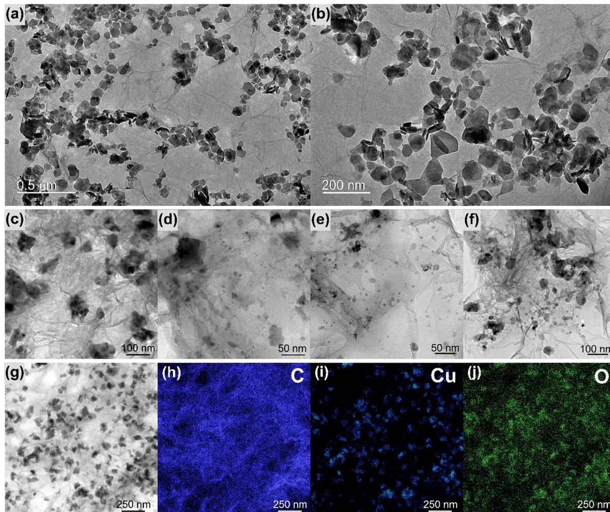
Fig. 4 Transmission electron microscopy images of the samples rGO/MoS<sub>2</sub> (a) and (b) and rGO/Cu<sub>x</sub>O (c)–(f). Energy dispersive spectroscopy mapping of rGO/Cu<sub>x</sub>O (g)–(j).
