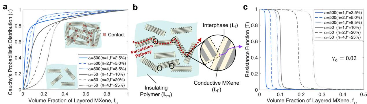
**Fig. 3** (a) Probability of interparticle contact formation of MXene clusters following Cauchy's cumulative probability function ( $\tau$ ) as the volume fraction ( $f_{\Omega}$ ) of layered MXene cluster increases. (b) Illustration of MXene clusters dispersed in a polymer with interparticle contacts forming a continuous pathway. (c) Overlapped interphase of neighboring MXene clusters leading to a local surge in functional property indicated by the drop in the resistance function ( $T$ ).
