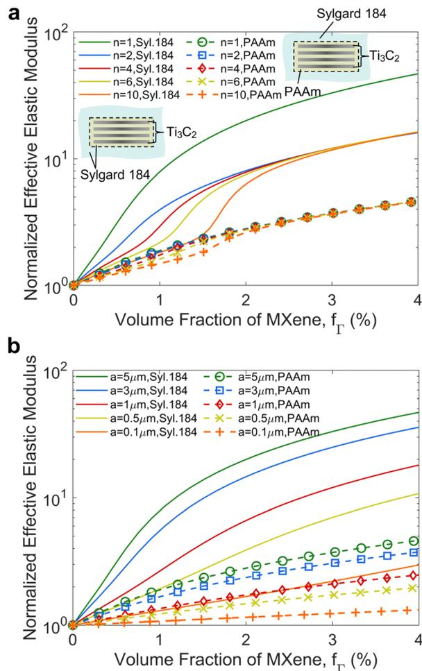
Fig. 6 (a) Suppressed stiffening behavior of Sylgard 184 composite with large (5  $\mu\text{m}$ ) single and multilayer MXenes when PAAm is used as the interphase. (b) Limited increase of elastic modulus in MXene-Sylgard 184 using smaller monolayer MXene flakes with gel interphase.
