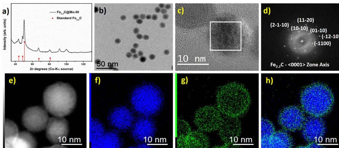
Fig. 3  $\text{Fe}_{2.2}\text{C}@$ Mo-IH NPs, (a) powder XRD pattern (ICDD: 00-036-1249, red vertical drop lines for standard  $\text{Fe}_{2.2}\text{C}$  pattern), (b) BF TEM micrograph, (c) HRTEM image, (d) FFT pattern derived from the white square marked zone of image c along (0001) zone axis, (e) STEM-HAADF image, (f)–(h) STEM-EDX elemental maps showing Fe in blue and Mo in green, and overlap of Fe and Mo maps.
