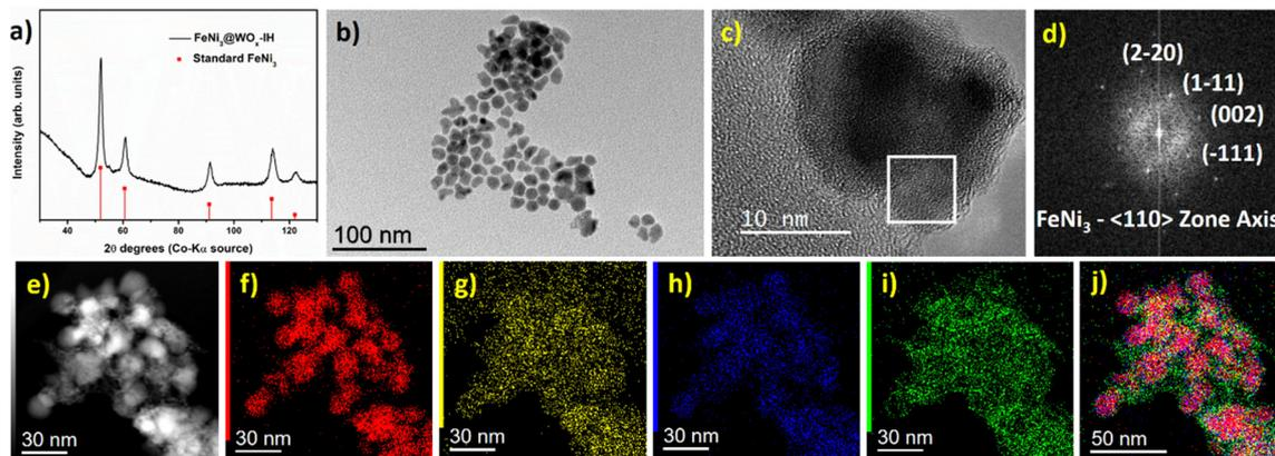
Fig. 6 FeNi<sub>3</sub>@W-IH NPs, (a) powder XRD pattern (ICDD: 00-038-0419, red vertical drop lines for standard FeNi<sub>3</sub>), (b) BF TEM micrograph, (c) HRTEM image and the corresponding FFT analysis (d) from the white square marked region, (e)–(j) STEM HAADF image and the respective STEM EDS elemental mapping shows Ni in red, O in yellow, Fe in blue, and W in green, and the overlap maps of W, Fe, and Ni.
