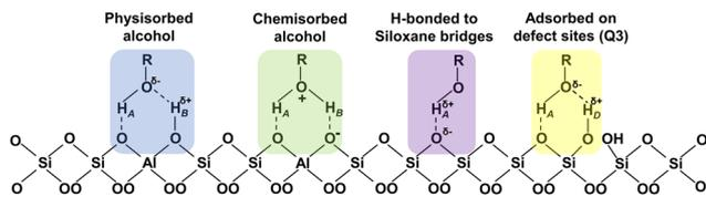
Fig. 4 Summary of the different modes of alcohol adsorption in zeolites namely physisorption (blue highlight) and chemisorption (green highlight) around a BAS, H-bonding to siloxane bridges (purple highlight) and adsorption at defect sites (yellow highlight).  $H_A$ ,  $H_B$ , and  $H_D$  respectively represent the  $^1\text{H}$  corresponding to the alcohol, Brønsted acid and defect sites (SiOH here, but can also be AlOH).
