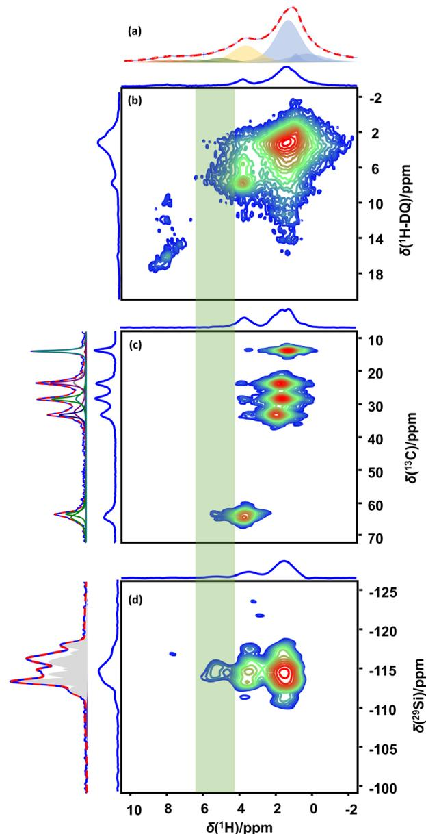
Fig. 3 Direct excitation  $^1\text{H}$  MAS NMR (a),  $^1\text{H}$ - $^1\text{H}$  DQ–SQ (b),  $^1\text{H}$ - $^{13}\text{C}$  CP-HETCOR (c),  $^1\text{H}$ - $^{29}\text{Si}$  CP-HETCOR (d) spectra of 1-pentanol adsorbed H-MFI-140. All the spectra were acquired at 253 K. Spectral decomposition of  $^1\text{H}$ ,  $^1\text{H}$ - $^{13}\text{C}$  CPMAS spectra and  $^{29}\text{Si}$  direct excitation spectra are presented along with the projections.
