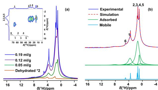
**Fig. 1** (a)  $^1\text{H}$  NMR spectra of MFI-140 exposed to different amounts of liquid 1-pentanol.  $^1\text{H}$ - $^{13}\text{C}$  CP-HETCOR spectrum (inset) aiding assignment of the resonances. (b) Spectral decomposition of the  $^1\text{H}$  NMR spectrum at a 1-pentanol dosage of 0.19 mL g<sup>-1</sup> on MFI-140. Adsorbed and mobile fractions are represented by the green and blue traces, respectively. All the spectra were acquired at 295 K.
