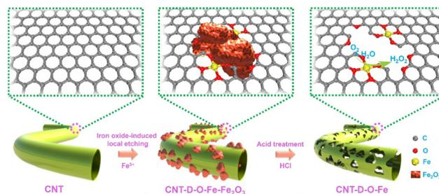
Fig. 1 Schematic of the preparation process of CNT-D-O-Fe.
