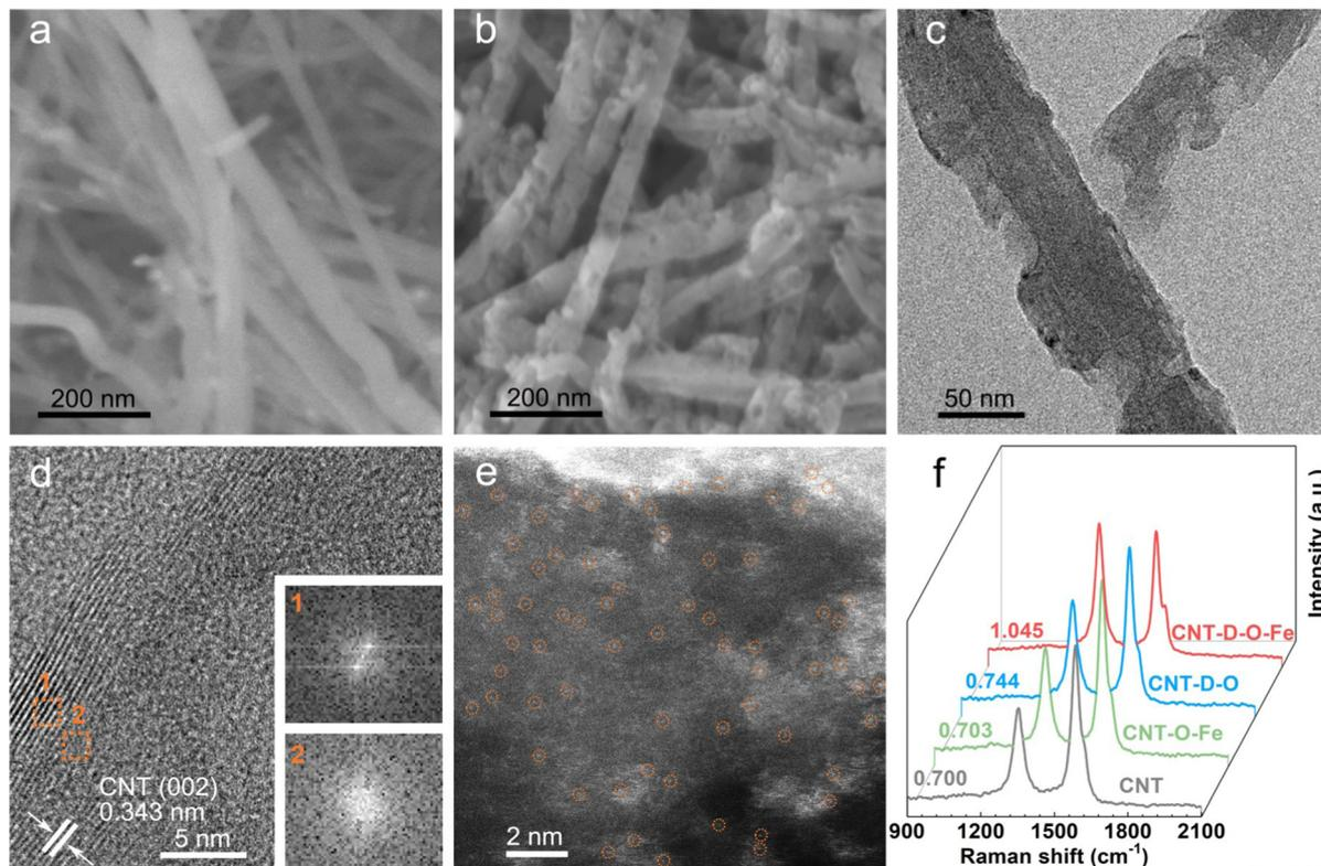
**Fig. 2** (a) SEM image of CNTs; (b) SEM and (c) TEM images of CNT-D-O-Fe; (d) HRTEM image of CNT-D-O-Fe and the corresponding fast Fourier transform (FFT) patterns (the inset) of the local CNT-D-O-Fe around the vacancy defects; (e) HAADF-STEM image of CNT-D-O-Fe; (f) Raman spectra of the samples.
