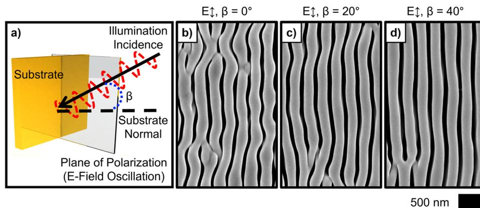
**Fig. 1** (a) Schematic illustration of electrode substrate illumination with linearly polarized light inclined in the plane of the polarization. (b)–(d) Representative SEMs of deposits generated with vertically polarized ( $E \uparrow$ )  $\lambda_{\text{avg}} = 626$  nm illumination with the indicated inclination ( $\beta$ ) from the substrate normal in the plane of the polarization.
