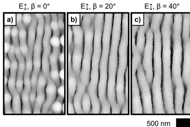
Fig. 3 Simulated deposit morphologies generated *via* growth modeling with vertically polarized ( $E \uparrow$ )  $\lambda_{\text{avg}} = 626$  nm illumination with the indicated inclination ( $\beta$ ) from the substrate normal in the plane of the polarization.
