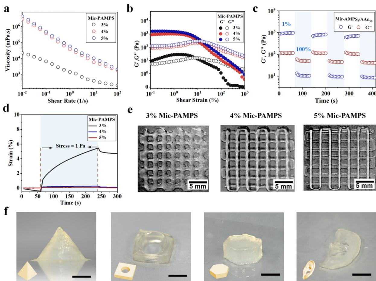
**Fig. 2** Jammed microgels for 3D printing. (a) Viscosity–frequency and (b) modulus–strain scans of mic-PAMPS/PAAC solutions with different microgel concentrations. (c) Self-healing of jammed 5 wt% PAMPS microgels swollen in 30% AAC solution. (d) Representative creep and recovery curves under 1 Pa load. Representative photos of printed (e) grids of microgel inks with different concentrations, and (f) pyramid, perforated tetrahedron, hexahedron and ear. Scale bar: 5 mm.
