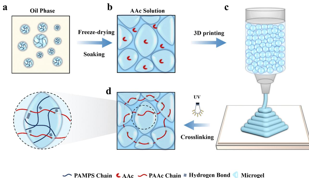
**Fig. 1** PAMPS microgels for 3D printing. (a) PAMPS microgels are prepared by inverse emulsion polymerization, (b) followed by soaking in AAc solution to produce a highly swollen and jammed microgel ink (c) for extrusion-based 3D printing various microstructures; (d) post-printing curing by UV light generates a PAAc network interpenetrating throughout the PAMPS microgels, yielding microgel-reinforced double network (MRDN) hydrogel constructs with different microstructures.
