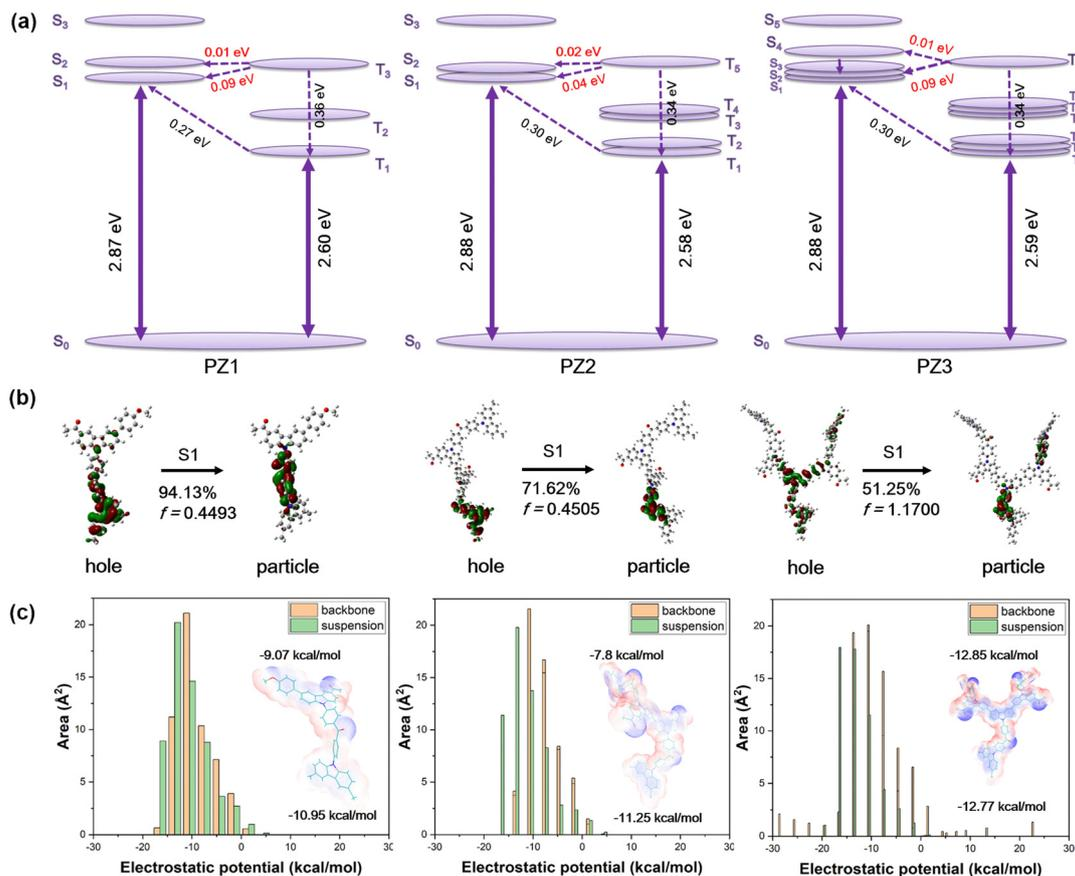
Fig. 2 (a) The calculated energy distributions. (b) The natural transition orbitals (NTOs) of  $S_1 \rightarrow S_0$ , and (c) the electrostatic potential (ESP) (inset: the ESP mapped molecular van der Waals surface) of the repeating units of **PZ1**, **PZ2** and **PZ3**, respectively.
