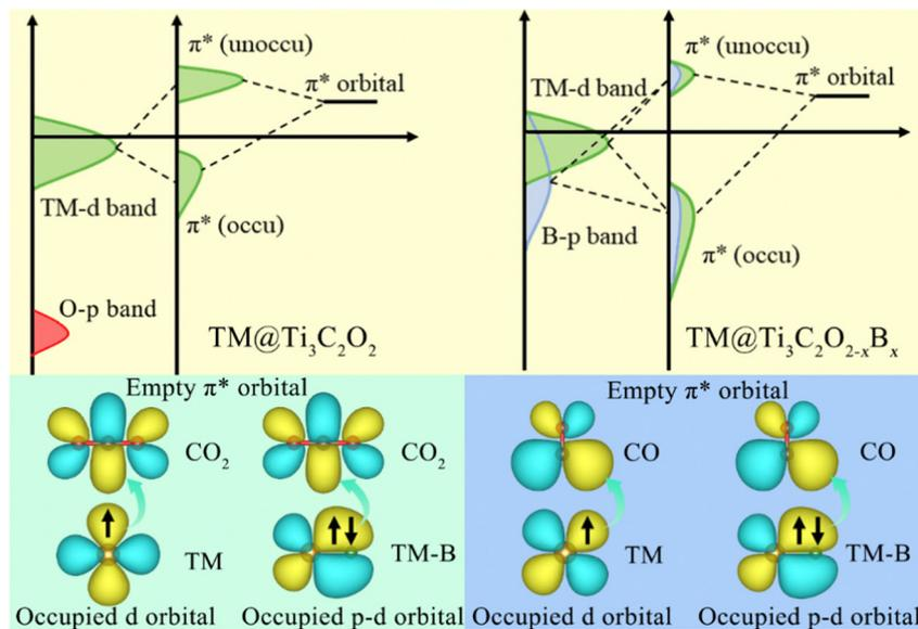
Fig. 7 Schematic diagrams of CO<sub>2</sub> molecule and CO intermediate activation mechanisms on TM@Ti<sub>3</sub>C<sub>2</sub>O<sub>2</sub> and TM@Ti<sub>3</sub>C<sub>2</sub>O<sub>2-x</sub>B<sub>x</sub>.
