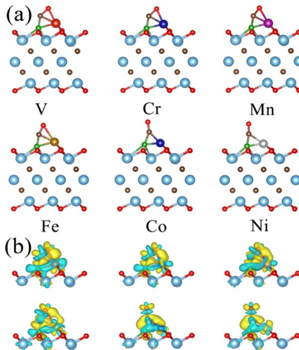
Fig. 4 (a) Optimized geometric structures of CO adsorbed on TM@Ti<sub>3</sub>C<sub>2</sub>O<sub>2-x</sub>B<sub>x</sub>. (b) Variation in the difference of charge density of TM@Ti<sub>3</sub>C<sub>2</sub>O<sub>2-x</sub>B<sub>x</sub> with a CO adsorption configuration. The yellow region denotes charge accumulation and the blue region indicates charge depletion, where the isosurface value is set to be 0.03 e Å<sup>-3</sup>.
