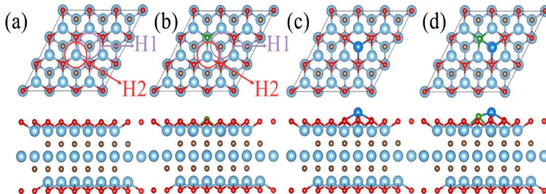
**Fig. 1** Optimized models of (a) pure  $\text{Ti}_3\text{C}_2\text{O}_2$  and (b)  $\text{Ti}_3\text{C}_2\text{O}_{2-x}\text{B}_x$ ; color scheme: Ti, cyan; C, brown; O, red; B, green; and TM, blue. Circles represent the possible sites of TM on  $\text{Ti}_3\text{C}_2\text{O}_2$ . Optimized structures of (c) pure  $\text{Ti}_3\text{C}_2\text{O}_2$  and (d)  $\text{Ti}_3\text{C}_2\text{O}_{2-x}\text{B}_x$  monolayer confining TM single atoms at the H1 site.
