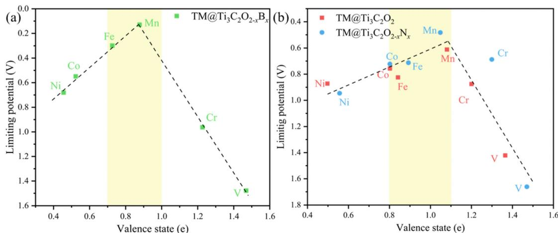
Fig. 10 The limiting potential as a function of the valence state of TM atoms fixed on (a)  $\text{Ti}_3\text{C}_2\text{O}_{2-x}\text{B}_x$  and (b)  $\text{Ti}_3\text{C}_2\text{O}_2$ ,  $\text{Ti}_3\text{C}_2\text{O}_{2-x}\text{N}_x$ .
