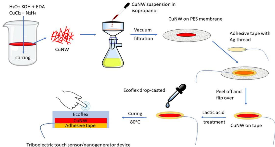
Fig. 1 Schematic for the fabrication of the CuNW-Ecoflex based single electrode TENG.
