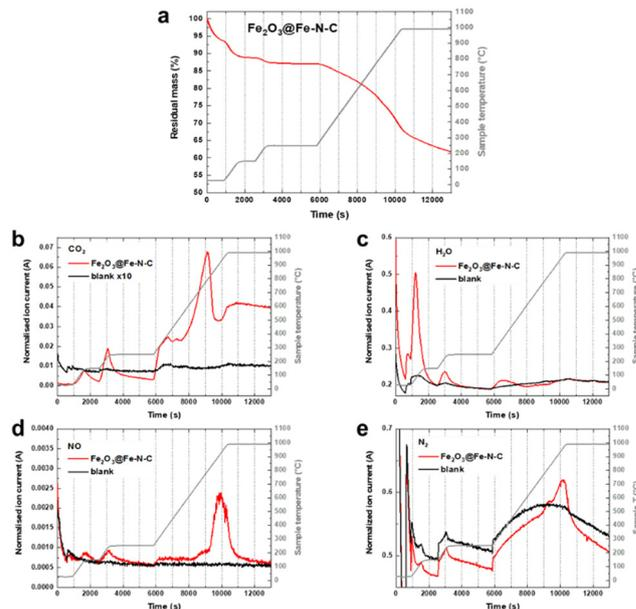
Fig. 4 (a) Results of the TGA-MS investigation of  $\text{Fe}_2\text{O}_3@/\text{Fe-N-C}$  upon heating to  $1000^\circ\text{C}$  under Ar atmosphere. TGA curve displaying the sample mass in percentage (red) and sample temperature (grey). (b)  $\text{CO}_2$ , (c)  $\text{H}_2\text{O}$ , (d) NO and (e)  $\text{N}_2$  MS signals for the sample (red) in comparison with a blank measurement where only the crucible without sample is employed (black). The sample temperature is displayed in grey.
