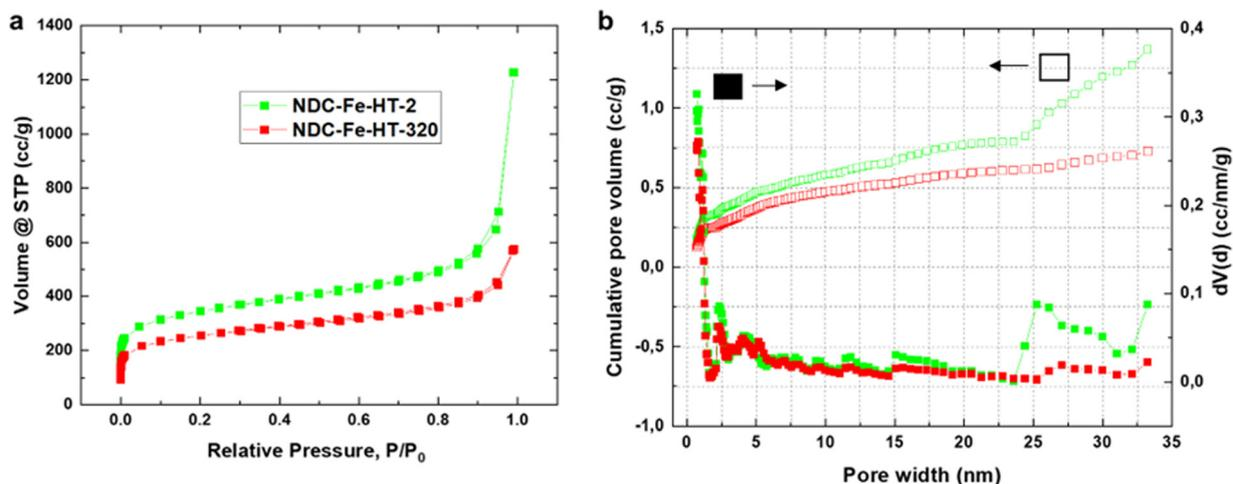
Fig. 3 (a) Isotherms of NDC-Fe-HT-X obtained from  $N_2$  sorption measurement. (b) The respective pore-size distribution from the adsorption branch employing the QSDFT model for slit and cylindrical pores.
