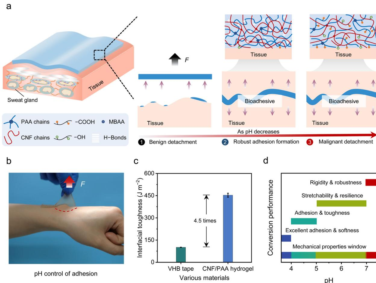
**Fig. 1** Design of a sweat-pH-triggered strong adhesive hydrogel. (a) Schematic illustrating the CNF/PAA hydrogel design. (b) Photographic image of the CNF/PAA hydrogel peeled from human skin. (c) Comparing the interfacial toughness of the CNF/PAA hydrogel and commercial VHB tape on sweaty skin with pH 4.5. (d) Mechanical and adhesive gradations of CNF/PAA hydrogels at various pH values.
