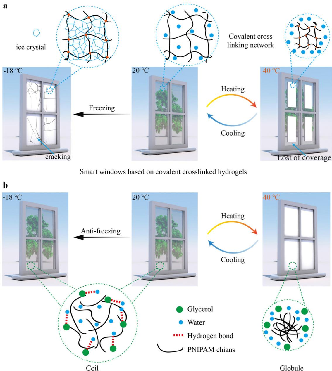
**Design strategy for smart windows with freezing tolerance, structural integrity and fast thermal responsive rate**
