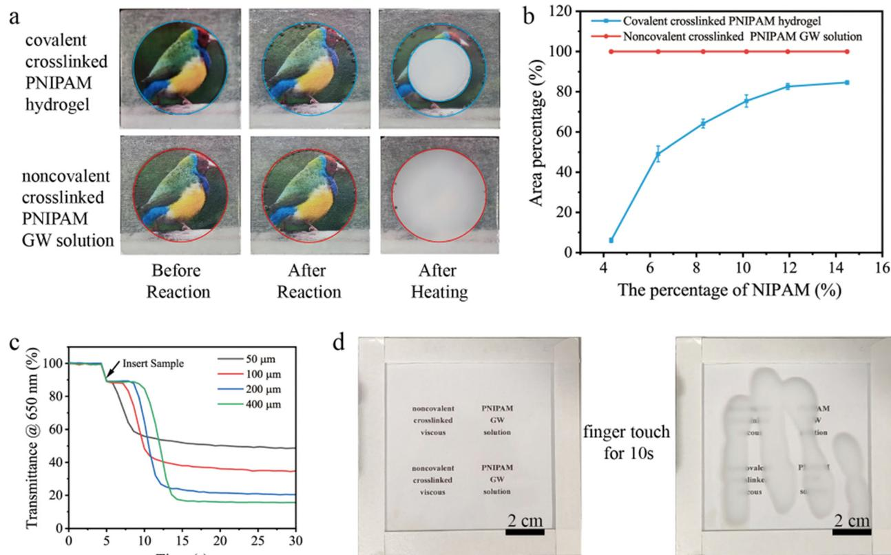
Fig. 3 (a) Photographs of smart windows in different states *via the in situ* polymerization. (b) The area percentage curves of the smart windows with the percentage of PNIPAM. (c) The thermal response curves of the noncovalent crosslinked viscous PNIPAM GW solutions with different thickness. (d) The phase transition photographs of the smart window triggered by finger touch. The thickness was  $400\text{ }\mu\text{m}$ .
