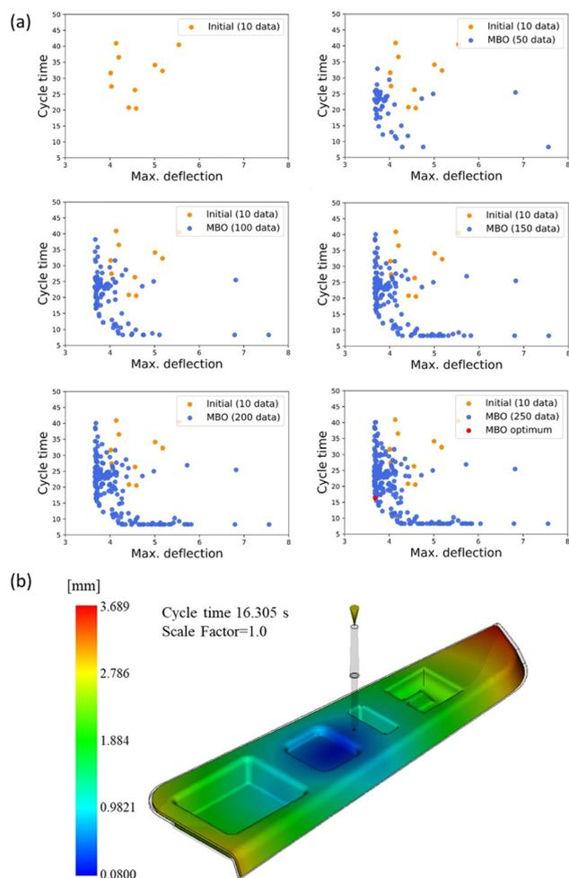
**Fig. 17** (a) Plot of the results of MBO for every 50 iterations. As the number of iterations increases, the Pareto line becomes more distinct. Design selection can be made from the data points on the plotted Pareto line that meet the specified condition (b) the deflection distribution for the optimized process parameter set comprised of cycle time and maximum deflection. Reproduction with permission from ref. 104. Copyright (2022) Springer Nature.
