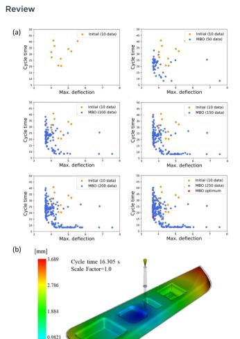
Fig. 17 (a) Plot of the results of MBO for every 50 iterations. As the number of iterations increases, the Pareto line becomes more distinct. Design selection can be made from the data points on the plotted Pareto line that meet the specified condition (b) the deflection distribution for the optimized process parameter set comprised of cycle time and maximum deflection. Reproduction with permission from ref. 104. Copyright (2022) Springer Nature
