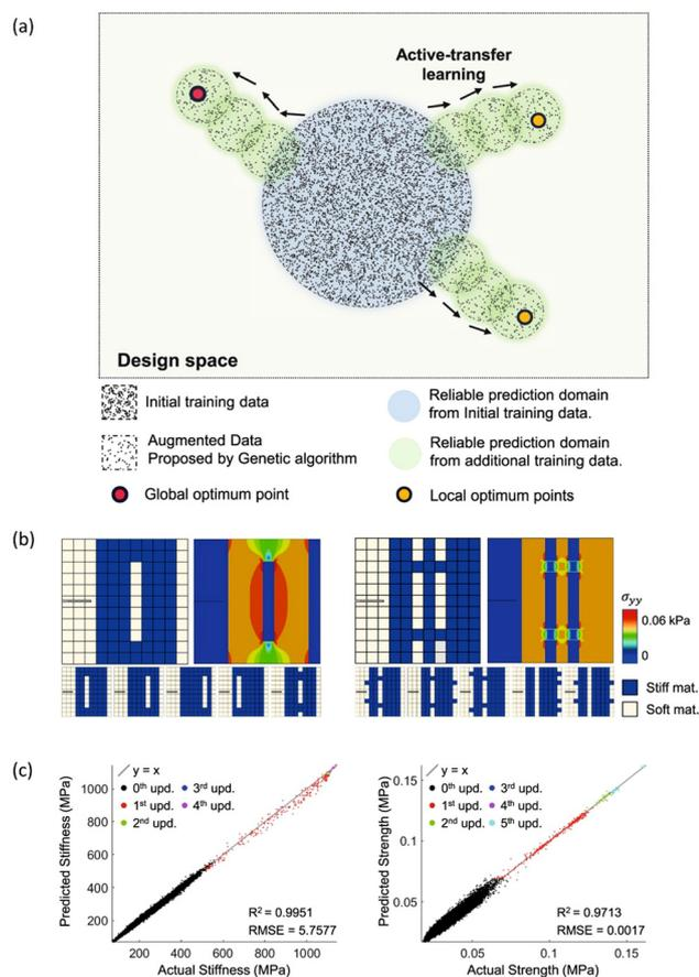
**Fig. 8** (a) Gradual expansion of reliable prediction domain through data addition using NN prediction-based genetic algorithm (b) optimized grid composite configuration for stiffness (Left) and strength (Right) (c) Increase in the stiffness (Left) and strength (Right) of grid composites on each update of the NN prediction-based genetic algorithm. From ref. 100, Licensed under CC BY 4.0.
