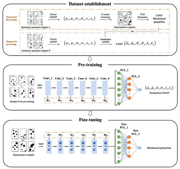
Fig. 14 Transfer learning workflow for micro structure-property prediction using CNN. CNN is pre-trained by ASDGF label, which is easier to compute, and CNN is fine-tuned by real mechanical properties. Reproduction with permission from ref. 127. Copyright (2021) Elsevier.
