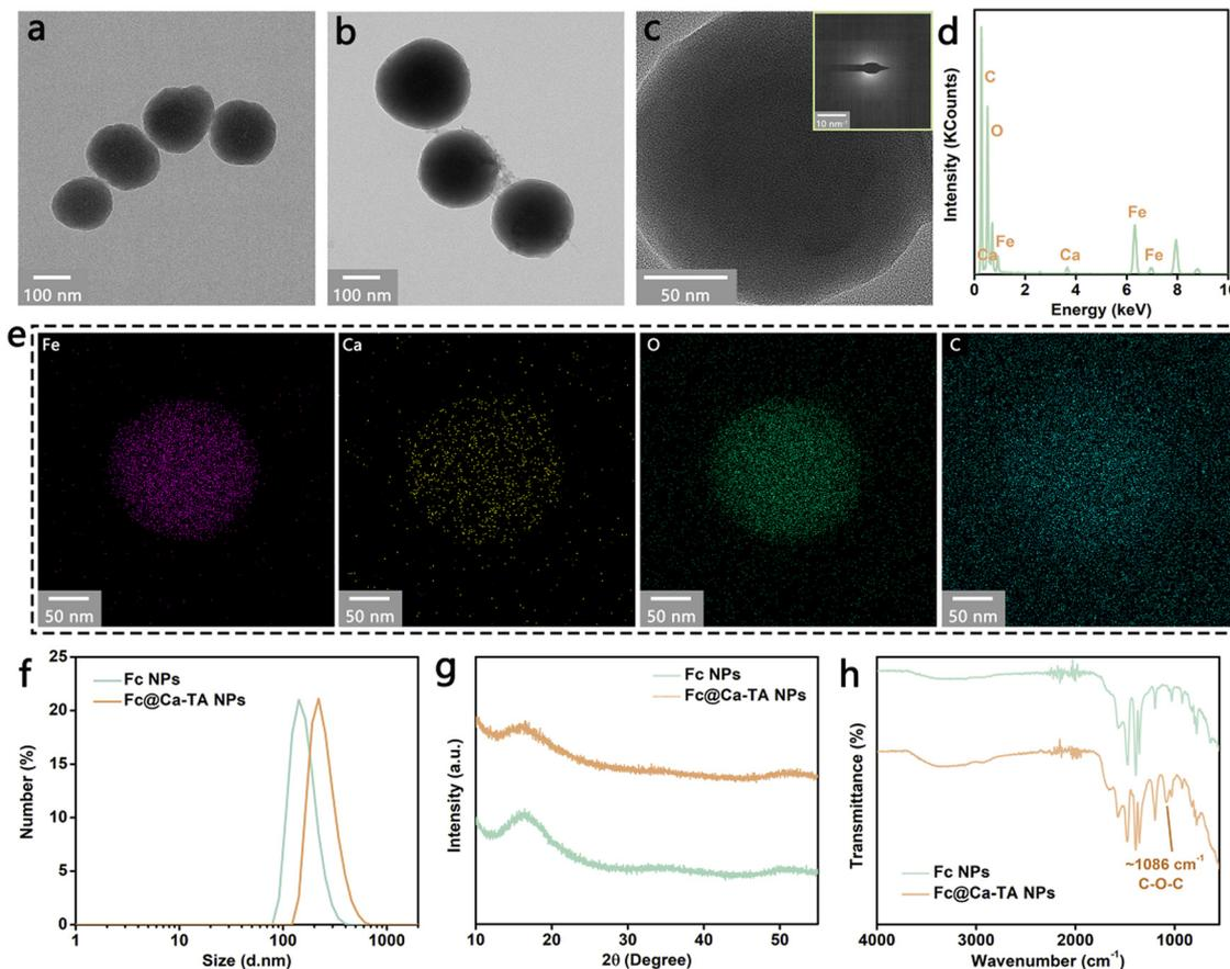
**Fig. 1** Preparation and characterization of Fc@Ca-TA NPs. (a and b) TEM images of Fc NPs and Fc@Ca-TA NPs. (c) High-magnification TEM image and SAED pattern of Fc@Ca-TA NPs. (d) EDS spectrum of Fc@Ca-TA NPs. (e) Elemental mapping of Fc@Ca-TA NPs. (f) DLS curves of Fc NPs and Fc@Ca-TA NPs. (g) XRD patterns of Fc NPs and Fc@Ca-TA NPs. (h) FT-IR spectrum of Fc NPs and Fc@Ca-TA NPs.
