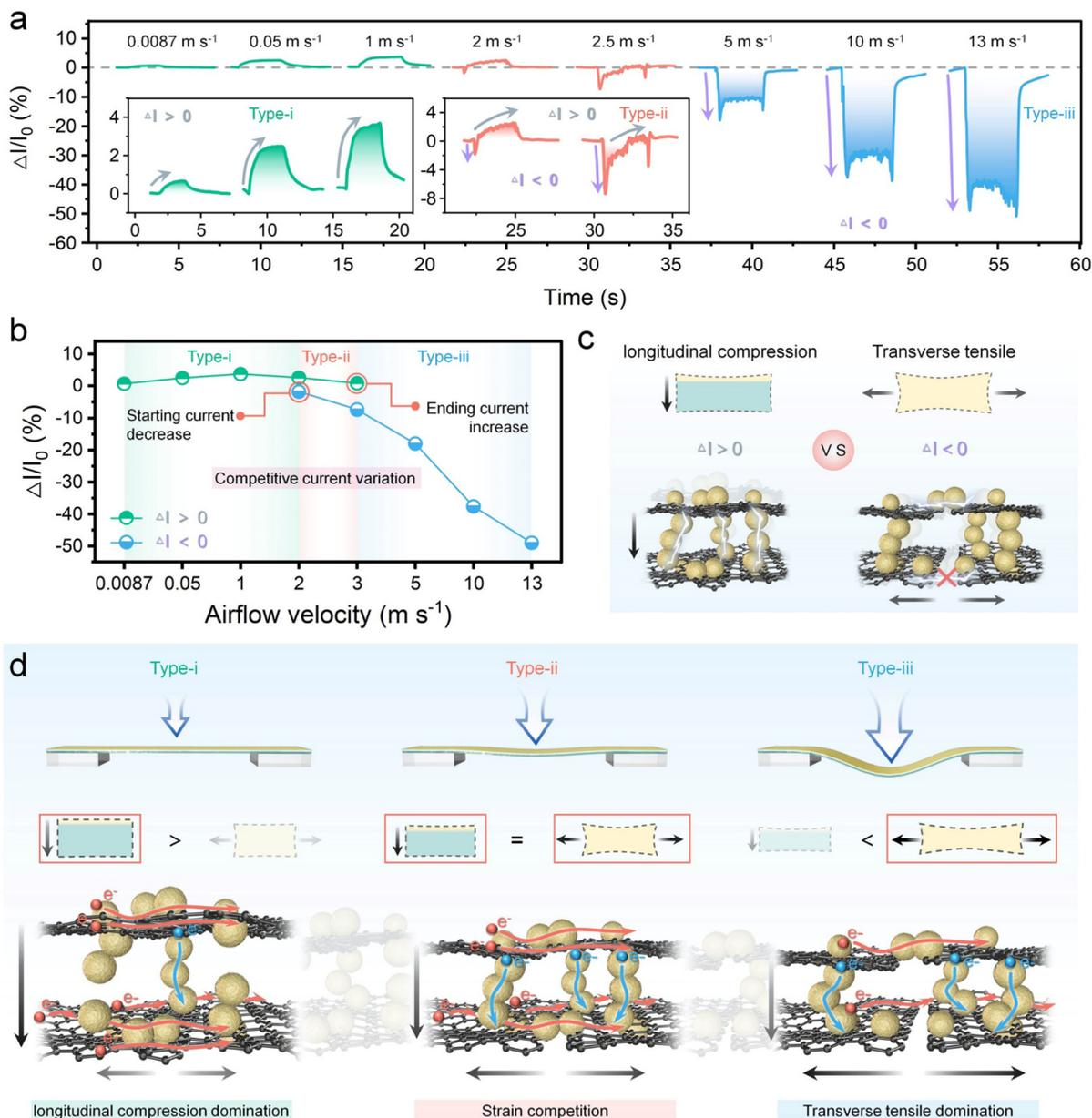
**Fig. 3** The characterization of the current response behavior. (a) Three types of current curves corresponding to different airflow velocities. (b) The trend of maximum current variation with the increase of airflow. (c) Schematic of the microscopic mechanism responsible for the increase and decrease of current. (d) Macroscopic and microscopic behaviors/mechanisms corresponding to the three types of current curves.
