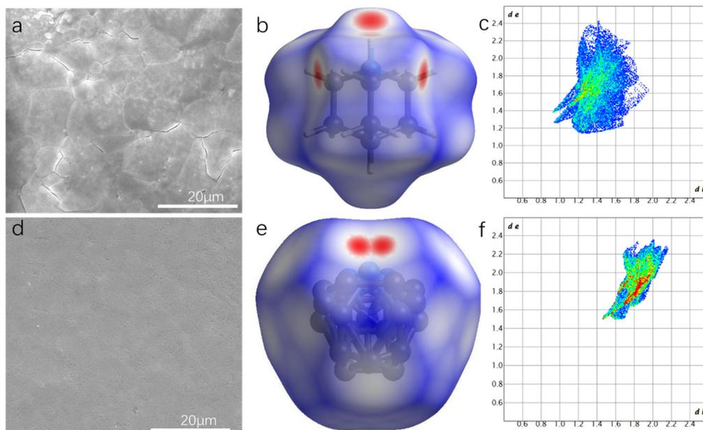
Fig. 3 Surface topography of different phases: (a and d) SEM image of the molecular ceramic obtained by applying pressure in the LTP and HTP; (b and e) Hirshfeld surfaces of HQReO<sub>4</sub> at 300 K and 350 K; (c and f) 2D fingerprint plots of HQReO<sub>4</sub> at 300 K and 350 K.
