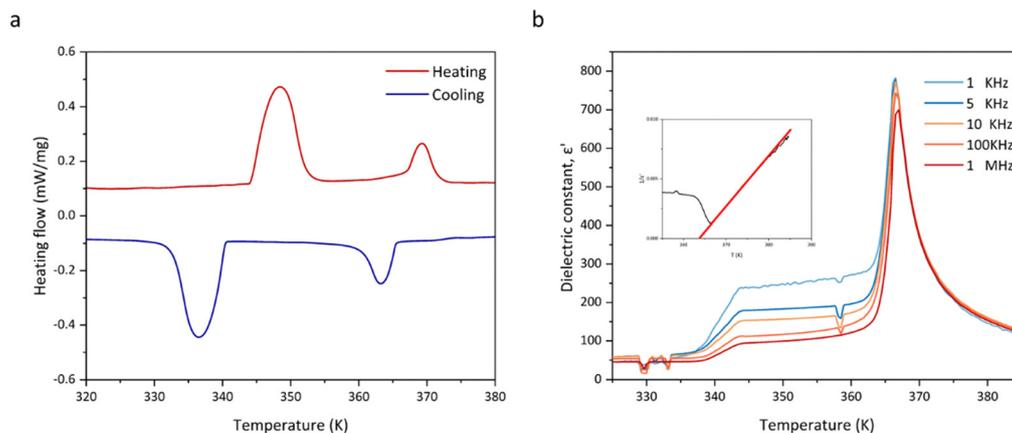
Fig. 2 Phase transition behaviours of HQReO<sub>4</sub>: (a) DSC curve exhibiting phase transitions of HQReO<sub>4</sub>; (b) dielectric constant at various frequencies. Inset is the linear fit to the Curie–Weiss law at 1 kHz of HQReO<sub>4</sub>.
