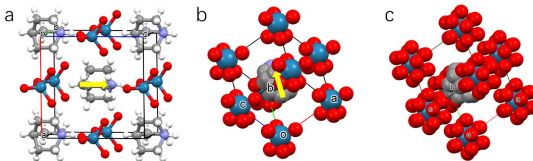
Fig. 1 Crystal structures of HQReO<sub>4</sub>. (a) Crystal structure in the LTP (300 K); the dipole moment of the quinuclidinium cation is indicated by the yellow arrow; (b) crystal structure in the ITP (350 K); (c) crystal structure in the HTP (380 K).
