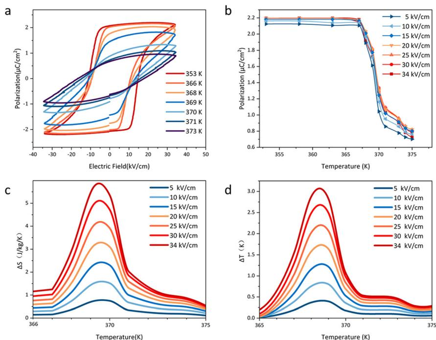
Fig. 4 (a) Polarization–electric field ( $P$ – $E$ ) hysteresis loops of the powder compacted bulk at different temperatures; (b) temperature-dependent polarization at different electric fields; (c) temperature-dependent isothermal entropy change  $\Delta S$  at different  $\Delta E$ ; (d) temperature-dependent adiabatic temperature change  $\Delta T$  at different  $\Delta E$ .
