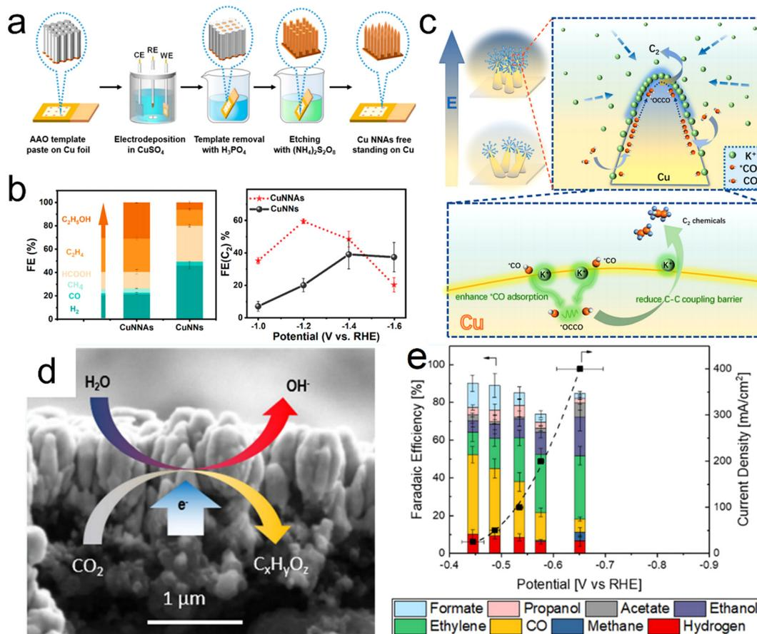
Fig. 5 (a) Diagram showing the synthesis of CuNNAs, (b) product distributions obtained from CuNNAs and CuNNs at  $-1.2$  V vs. RHE together with  $FE(C_{2+})$  values at different potentials, (c) diagram showing  $C_{2+}$  formation on the single tip of a CuNNA. (d and e) Electron beam image of a Cu catalyst and corresponding FE values at different potentials. Reproduction with permission from ref. 97 and 98, Copyright 2022, American Chemical Society.
