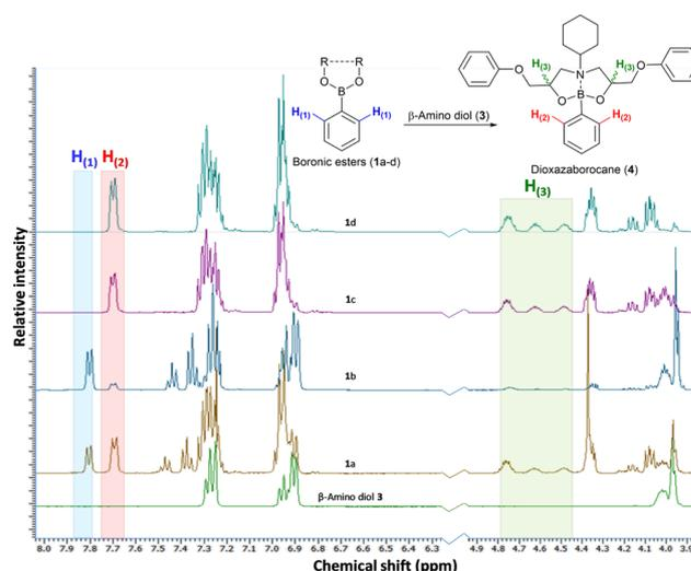
Fig. 1 <sup>1</sup>H-NMR analysis of the reaction mixtures of boronic esters **1a–d** with model  $\beta$ -amino diol **3**. Hydrogen environments of interest are indicated as according to the colours H-atom ( $H^1$ ,  $H^2$  and  $H^3$ ) labelled on both the molecule structures and spectra.
