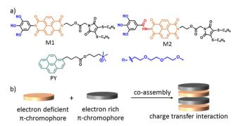
Scheme 1 (a) Structure of M1, M2 and PY, (b) Schematic representation of  $\pi - \pi$  interaction mediated charge transfer complex formation.
