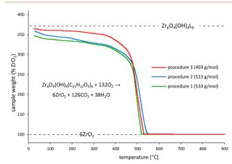
Fig. 3 TGA curves (relative to ZrO2) obtained from UiO-68-CHO samples synthesized according to procedures 1, 2 and 3. The position of the theoretical TGA plateau for defect-free UiO-68-CHO is marked with the dashed line labelled 'Zr<sub>6</sub>O<sub>4</sub>(OH)<sub>4</sub>L<sub>6</sub>'.
