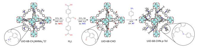
Fig. 1 Solvothermal synthesis of UiO-68-CHO and UiO-68-CH₂NHMe₂+Cl⁻, and post-synthetic modification of UiO-68-CHO with 4-methylaniline. BA = benzoic acid, DMF = N,N-dimethylformamide, ACN = acetonitrile.
