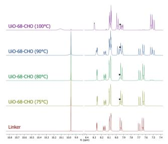
Fig. 2 <sup>1</sup>H NMR spectra of linker H<sub>2</sub>L (bottom) and the digested samples of UiO-68-CHO synthesized at temperatures ranging from 75 °C to 100 °C. Signals from DMF are marked with stars.
