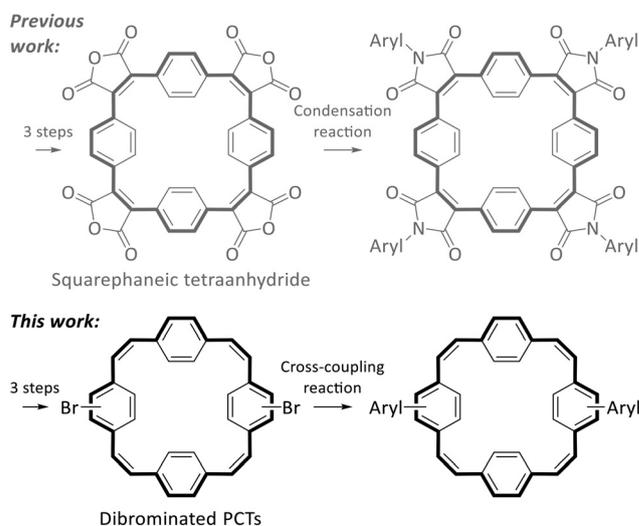
**Scheme 2** Previous work: squarephaneic tetraanhydride as a building block for the synthesis of molecules with cross-conjugated imide groups between the PCT core and the aryl groups. This work: dibrominated PCTs as building blocks for the synthesis of molecules with linear conjugation between the PCT core and the aryl groups.
