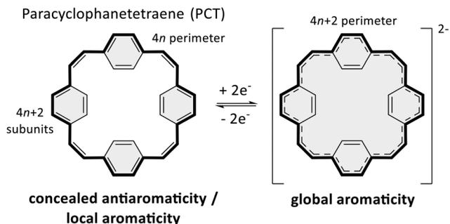
**Scheme 1** Redox reaction and aromaticity switching of paracyclophanetetraene (PCT; grey shadings indicate aromaticity). In the neutral state, the antiaromaticity of the formal macrocyclic 24 ( $4n$ )  $\pi$ -electron system (bold bonds) is concealed by the locally aromatic subunits, but the dianion can still become globally aromatic.
