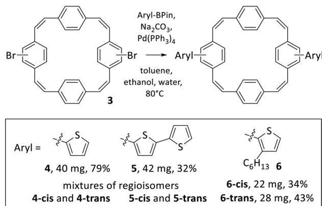
**Scheme 4** Suzuki cross-coupling reactions of the mixture of dibrominated PCT isomers **3** and the respective boronic acid pinacol esters (Aryl-BPin), yielding dithienyl-substituted PCT **4** and bis(bithienyl)-substituted PCT **5** as mixtures of isomers and bis(3-hexylthienyl)-substituted PCT **6** as separated isomers **6-cis** and **6-trans** following purification by recycling preparative GPC.
