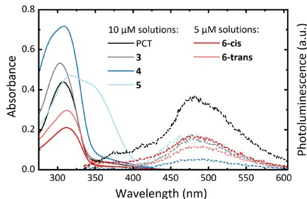
Fig. 2 UV-vis absorption (solid lines) and photoluminescence spectra (dashed lines) of the macrocycles in  $\text{CHCl}_3$  solution (approx. 5 and 10  $\mu\text{M}$ ). For recording the PL spectra, the macrocycles were excited at their absorption maximum wavelengths.
