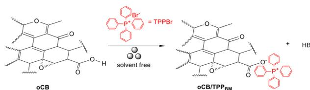
**Scheme 1** Ionic functionalization of oCB with TPPBr promoted by ball milling under solvent-free conditions.
