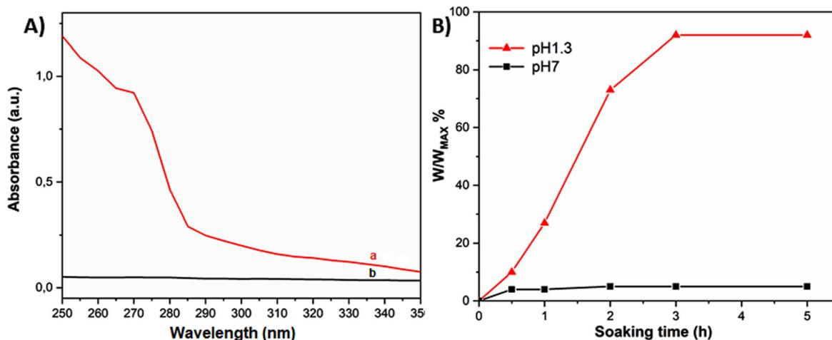
Fig. 4 (A) UV measurements in the spectral range 250–350 nm, in the neutral aqueous solution (b) and acidic solution (a) after 5 h of soaking time; (B) TPP<sup>+</sup> kinetic release from oCB/TPP<sub>BM1/1</sub> in neutral saline solution (pH = 7 black curve, squares) and in acidic solution (pH = 1.3, red curve, triangles) expressed as a percentage of the long term release.
