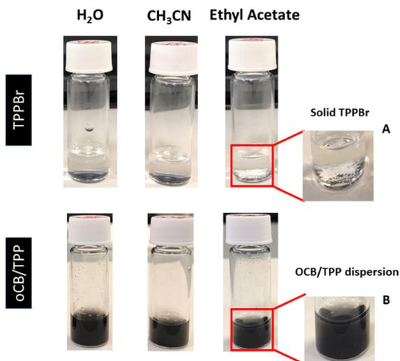
**Fig. 5** TPPBr and oCB/TPP in water, acetonitrile, and ethyl acetate solution 5 mg mL<sup>-1</sup>, after 5 min of sonication and 30 minutes of storage. Inset A and B: solid TPPBr as sediment and oCB/TPP dispersion in ethyl acetate, respectively.
