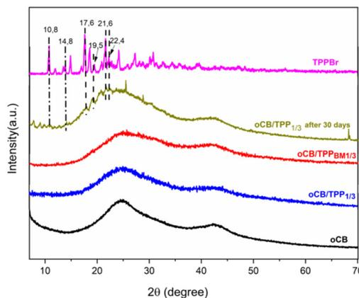
Fig. 2 X-ray diffraction patterns of oCB (black), oCB/TPP<sub>1/3</sub> (blue) as obtained in solution, oCB/TPPBm<sub>1/3</sub> as obtained by ball milling (red), oCB/TPP<sub>1/3</sub> after 30 days (olive), and TPPBr salt (pink).
