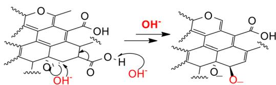
Scheme 2 Proposed mechanism of decarboxylation and epoxy ring opening in alkaline solution.
