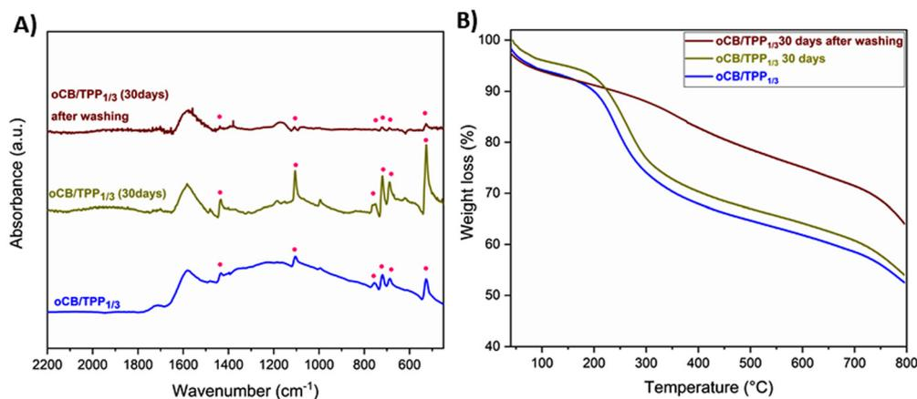
Fig. 3 FTIR spectra (A) and TGA scans (B) of oCB/TPP<sub>1/3</sub> (blue), oCB/TPP<sub>1/3</sub> after 30 days (green), and oCB/TPP<sub>1/3</sub> after 30 days and after washing (brown).
