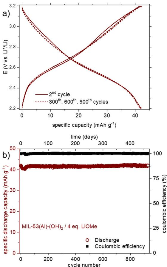
**Fig. 8** a) Potential vs. specific capacity curves for the lithiation product from MIL-53(Al)-(OH)<sub>2</sub> and LiOMe–MeOH/THF. Plain lines correspond to the 2<sup>nd</sup> cycle; dashed lines to the 300<sup>th</sup>, 600<sup>th</sup> and 900<sup>th</sup> cycles; b) capacity retention and coulombic efficiency for the lithiation product from MIL-53(Al)-(OH)<sub>2</sub> and 4 eq. of LiOMe (electrolyte: 1 M LiClO<sub>4</sub> in PC; potential range: 2.2–3.2 V vs. Li<sup>+</sup>/Li).
