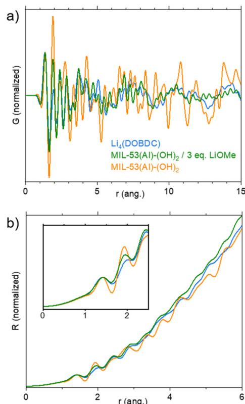
**Fig. 4** Characterisation of the reaction product between MIL-53(Al)-(OH)<sub>2</sub> and 3 eq. of LiOMe in MeOH/THF by X-ray total scattering experiments. a) Reduced pair distribution function  $G(r)$ ; b) radial distribution function  $R(r)$  (inset: zoom on the 0–2.5 ang. region). Data related to dry MIL-53(Al)-(OH)<sub>2</sub>, Li<sub>4</sub>(DOBDC), and the lithiation product from LiOMe–MeOH/THF, are shown in orange, blue and green, respectively.
