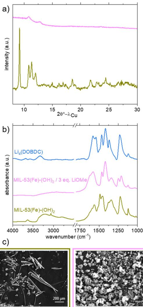
**Fig. 5** Characterisation of  $\text{MIL-53}(\text{Fe})-(\text{OH})_2$  and its lithiated product from LiOMe in MeOH/THF. a) PXRD patterns ( $\lambda = 1.5406\text{ \AA}$ ); b) IR spectra; c) SEM pictures. Data related to dry  $\text{MIL-53}(\text{Fe})-(\text{OH})_2$ ,  $\text{Li}_4(\text{DOBDC})$  and the lithiation product are shown in khaki, blue and pink, respectively.
