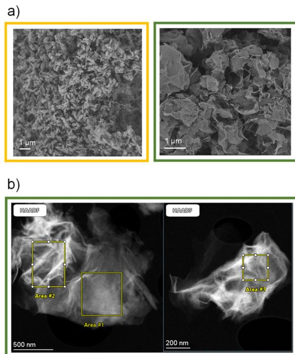
**Fig. 3** Characterization of the reaction product between MIL-53(Al)-(OH)<sub>2</sub> and 3 eq. of LiOMe in MeOH/THF. a) SEM pictures of the pristine solid (left) and the lithiated solid (right); b) STEM pictures of the lithiated product. Areas used for the EDX analyses provided in Table 1 are also shown.
