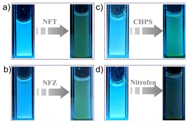
**Fig. 2** Photographs of the emission intensity changes of **iMOF-14C** in water under UV-vis light ( $\lambda = 350$  nm) upon the addition of an (a) aqueous solution of NFT, (b) aqueous solution of NFZ, (c) aqueous solution of CHPS and (d) aqueous solution of nitrofen, each showing rapid quenching of PL emission intensity.
