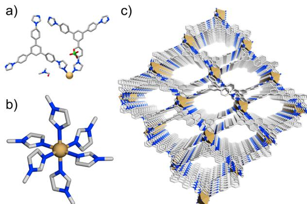
**Fig. 1** The structural representation of **iMOF-14C** illustrating (a) the asymmetric unit and (b) the coordination environment of Cd(II); (c) the view along the *c* axis, showing one-dimensional ultramicroporous (<7 Å) channels that sustain the MOF (colour code: grey – C, blue – N, dark yellow – Cd, red – O, green – Cl; ClO<sub>4</sub><sup>−</sup>, the solvent molecules and hydrogen atoms are omitted for clarity in figures b and c).
