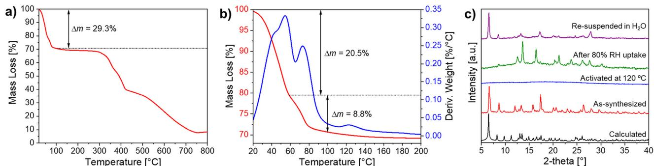
**Fig. 2** Thermogravimetric and PXRD characterizations of Ni-ZW-MOF. a) Full TGA profile under  $N_2$  atmosphere ranging 20–800 °C; b) TGA (red) and DTG (blue) profiles in the <200 °C range; and c) PXRD analysis after different water adsorption and desorption processes.
