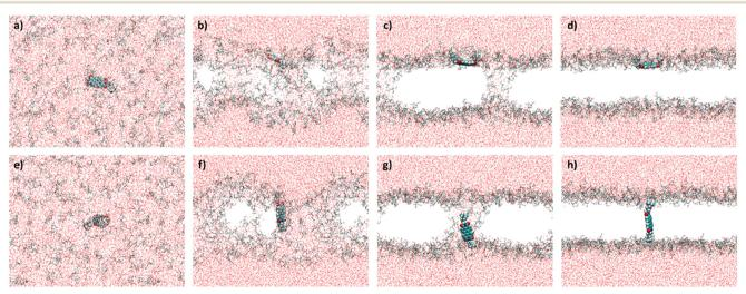
Fig. 5 Stages of the membrane assembly in the simulations. a-d) Parallel insertion of [1]<sup>2+</sup> (62-81%, see Table 3); e-h) transmembrane insertion of [1]<sup>2+</sup> (19–38%, see Table 3). Color code: red = oxygen, white = hydrogen, blue = nitrogen, yellow = phosphorus, and turquois = carbon. The alkyl tails of the lipid bilayer are omitted for clarity.
