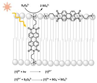
Fig. 1 Light absorption by [1]<sup>2+</sup> is followed by photooxidation of [1]<sup>2+</sup> by persulfate; equations of initial light-driven reactions are included.
