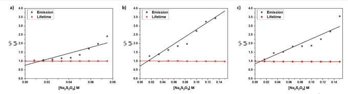
Fig. 7 Stern-Volmer quenching experiments for different systems: a) acetonitrile/water 1:1 (V:V), b) DOPG: (14:0 PEG2000 PE): [1]<sup>2+</sup> = 100:1:1 liposomes in phosphate buffer (10 mM, pH 7.0) without size exclusion chromatography, c) DOPG: (14:0 PEG2000 PE): [1]<sup>2+</sup> = 100:1:1 liposomes in phosphate buffer (10 mM, pH 7.0) after size exclusion chromatography.
