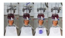
Fig. 14 Images of the water separation tests using coated nylon membrane which allows water to be removed whilst simultaneously retaining Jet A-1 fuel. In the case with no membrane present the fuel freely passes through.
