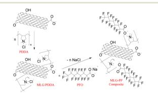
Scheme 1 Synthesis of MLG-PP composite consisting of a two-step process involving adsorption of PDDA onto MLG followed by complexation of PFO with the PDDA/MLG mixture.
