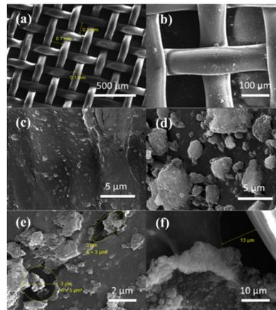
**Fig. 11** SEM images of (a) uncoated nylon at a magnification of 125 $\times$ ; and coated nylon at magnifications of (b) 415 $\times$  (c) 10.38k $\times$  (d) 10.39k $\times$  (e) 20.75k $\times$  and (f) 4.15k $\times$ .
