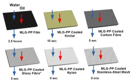
**Fig. 2** Schematic outlining the passage of water and oil through MLG-PP film and coated substrates. Water passage is represented by blue arrows, whilst red arrows represent silicone oil passage. \*Note: on some occasions, the glass fibre coated substrate allowed oil penetration after 2 hours.
