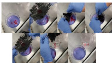
Fig. 13 Photographs outlining how coated carbon fibre supported by stainless steel mesh was utilised to remove silicone oil from the surface of water.
