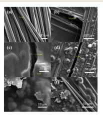
Fig. 9 SEM images of (a) uncoated carbon fibre at a magnification of 1.38k× and coated carbon fibre at magnifications of (b) 461× (c) 2.08k× (d) 830k× (e) 4.15k× and (f) 1.04k×.
