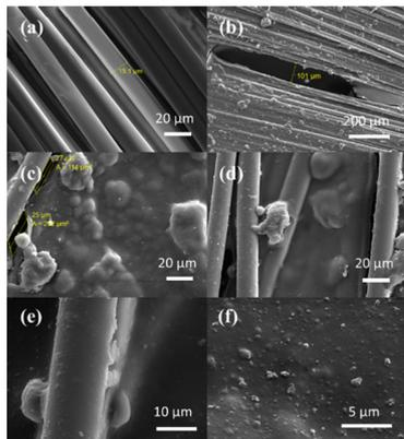
**Fig. 10** SEM images of (a) uncoated glass fibre at a magnification of 1.38k $\times$ ; and coated glass fibre at magnifications of (b) 208 $\times$  (c) 1.38k $\times$  (d) 1.38k $\times$  (e) 4.15k $\times$  and (f) 10.38k $\times$ .
