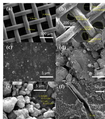
**Fig. 12** SEM images of (a) uncoated stainless steel mesh at a magnification of 106 $\times$ ; and coated stainless steel mesh at magnifications of (b) 208 $\times$  (c) 10.38k $\times$  (d) 10.38k $\times$  (e) 9.96k $\times$  and (f) 692 $\times$ .
