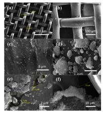
Fig. 11 SEM images of (a) uncoated nylon at a magnification of 125×; and coated nylon at magnifications of (b) 415× (c) 10.38k× (d) 10.39k× (e) 20.75k× and (f) 4.15k×.
