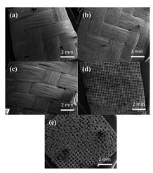
Fig. 7 SEM images obtained in wide field mode of coated (a) Keylar (b) carbon fibre (c) glass fibre (d) nylon and (e) stainless steel mesh at magnifications of 20x.
