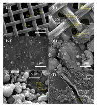
Fig. 12 SEM images of (a) uncoated stainless steel mesh at a magnification of 106x; and coated stainless steel mesh at magnifications of (b)  $208\times$  (c)  $10.38k\times$  (d)  $10.38k\times$  (e)  $9.96k\times$  and (f) 692×.
