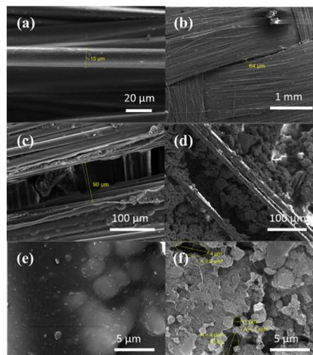
Fig. 8 SEM images of (a) uncoated Kevlar at a magnification of 1.73k $\times$  and coated Kevlar at magnifications of (b) 56 $\times$  (c) 589 $\times$  (d) 519 $\times$  (e) 10.38k $\times$  and (f) 10.38k $\times$ .
