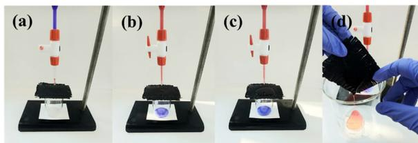
**Fig. 1** Coated carbon fibre at various stages during oil/water passage tests (a) before liquid deposition, (b) water penetrated coated carbon fibre after approximately 5 seconds, (c) oil remained on top for at least 3 weeks and (d) silicone oil could easily be poured off the surface.
