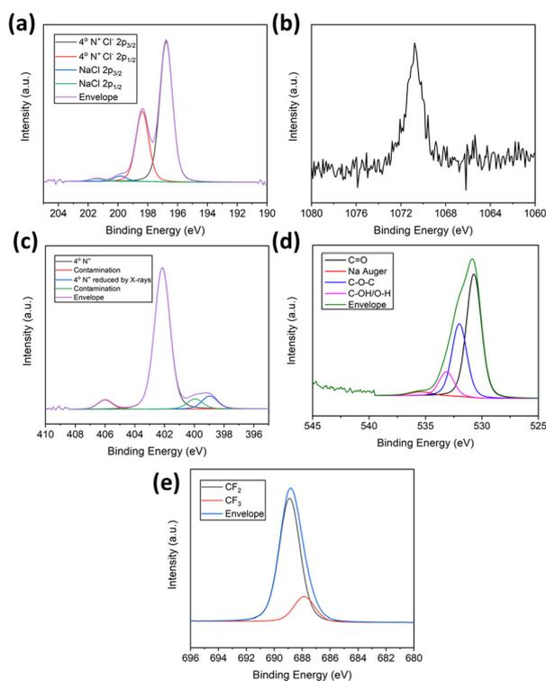
Fig. 5 High-resolution deconvoluted spectra for MLG-PP composite showing (a) Cl 2p orbital (b) Na 1s orbital (c) N 1s (d) O 1s (e) F 1s.
