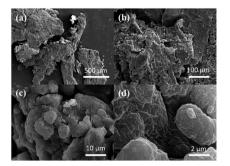
Fig. 6 SEM image of MLG–PP composite at magnifications of (a)  $105 \times (b) 415 \times (c) 4.15 \times and (d) 20.76 \times .$
