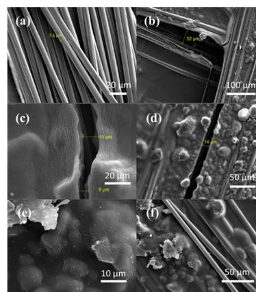
Fig. 9 SEM images of (a) uncoated carbon fibre at a magnification of 1.38k $\times$  and coated carbon fibre at magnifications of (b) 461 $\times$  (c) 2.08k $\times$  (d) 830k $\times$  (e) 4.15k $\times$  and (f) 1.04k $\times$ .
