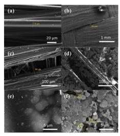
Fig. 8 SEM images of (a) uncoated Kevlar at a magnification of 1.73k× and coated Kevlar at magnifications of (b)  $56\times$  (c)  $589\times$  (d)  $519\times$  (e) 10.38k× and (f) 10.38k×.
