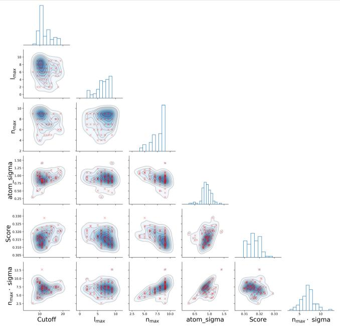
Fig. 3 There are no simple (cor)relations between the different SOAP parameters. Correlations between the SOAP parameters for the all-all SOAP, as well as the score. The scatter plots refer to the best set of SOAP parameters obtained for 96 statistically independent GA.
