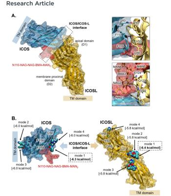
Fig. 4 ICOS/ICOSL structures. (A) ICOS/ICOSL complex with highlighted key residues for interactions formed at the ICOS/ICOSL interface. The structure of ICOS is shown in blue, ICOSL is shown in yellow, and the N110-NAG-NAG-BMA-MAN2 oligosaccharide chain is shown in red. (B) The highest-scored position of AG-120 in ICOS and ICOSL obtained in docking studies. Values provided in brackets correspond to binding affinity determined based on the scoring function.
