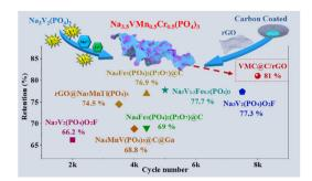
Hierarchical cathode constructed by carbon coated Na<sub>3.5</sub>VMn<sub>0.5</sub>Cr<sub>0.5</sub>(PO<sub>4</sub>)<sub>3</sub> nanoparticles on rGO for high-capacity and long-cycle life sodium storage
