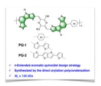
6H-[1,2,5]Thiadiazolo[3,4-e]thieno[3,2-b]indoleflanked para-azaguinodimethane based aromatic-quinoidal polymer semiconductors with high molecular weights synthesized via direct arylation polycondensation
