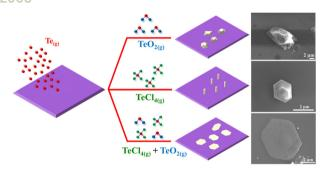
Chloride-assisted synthesis of tellurene directly on SiO<sub>2</sub>/Si substrates: growth mechanism, thermal properties, and device applications
