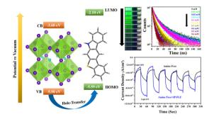
Surface engineering of CsPbBr<sub>3</sub> perovskite nanocrystals: hole transfer dynamics and enhanced photocurrent response using a novel organic molecule
