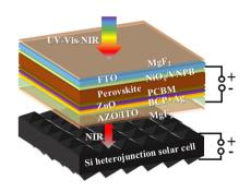
Designed multi-layer buffer for high-performance semitransparent wide-bandgap perovskite solar cells
