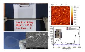
One-step fabrication of highly stable, durable, adhesion enhanced, flexible, transparent conducting films based on silver nanowires and neutralized PEDOT:PSS
