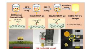
High mechanically enhanced and degradable polybenzoxazine/polyhexahydrotriazine IPN aerogels by atmospheric drying
