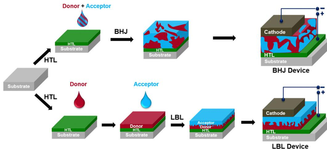
Fig. 1 Schematic representation of the preparation of BHJ and LBL OSCs.
