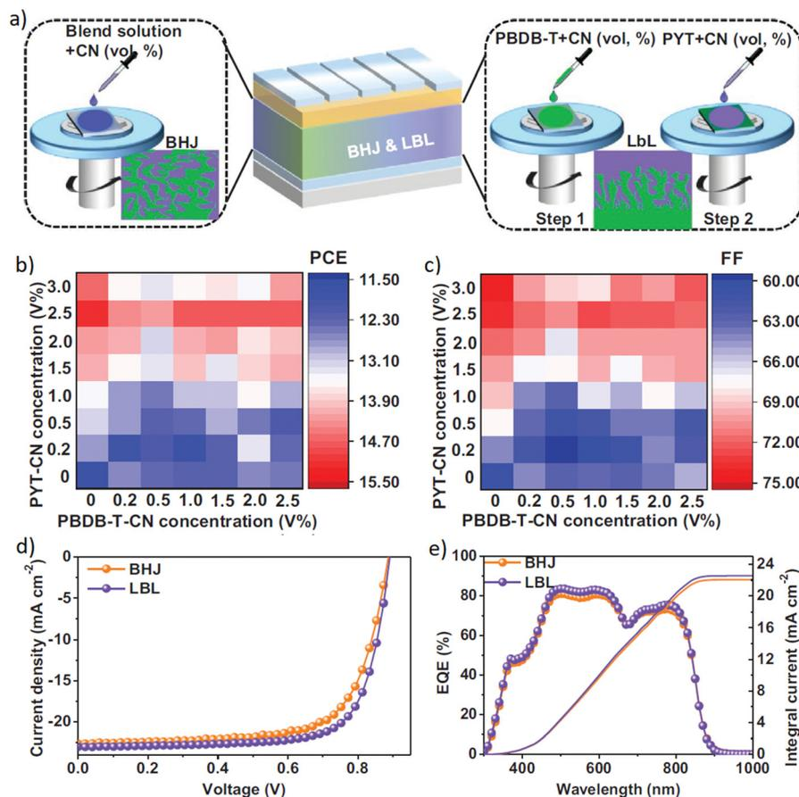
Fig. 15 (a) Representation of BHJ and LBL OSC processing. (b) PCE and (c) FF of the PBDB-T/PYT LBL all-polymer OSCs as a function of 1-CN content for each layer. (d)  $J$ - $V$  characteristics and (e) the equivalent EQE spectra for the optimized devices. Reprinted with permission from ref. 177. Copyright 2021, Wiley-VCH.
