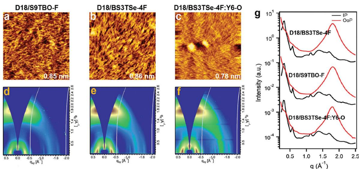
Fig. 11 (a)–(c) AFM height images ( $2 \times 2 \mu\text{m}^2$ ) and (d)–(f) 2D-GIWAXS patterns for the binary and ternary PMHJ films. (g) Corresponding GIWAXS line-cut profiles. Reprinted with permission from ref. 125. Copyright 2022, Wiley-VCH.
