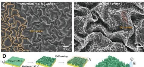
Rinsing by Hierarchical wrinkle Fig. 5 Approaches employed to minimise the accumulation of gas bubbles at the electrocatalyst surface (A) and (B)  $CoSe_2/MoSe_2$  heterostructures, reprinted with permission from the Royal Society of Chemistry, Chen et al. 118 and (C) wrinkled  $VMoS_2$  and (D) schematic of the wrinkling procedure, reprinted with permission from the American Chemical Society, Jung et al. 122
