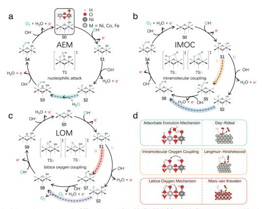
Fig. 4 Schematic of the reaction mechanisms for OER on Ni-based LDHs, (a) AEM, (b) IMOC, and (c) LOM mechanisms and (d) their association with heterogeneous catalysis mechanisms, taken from Wang  ${\it et al.}^{97}$
