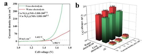
Fig. 6 (a) LSV curves and (b) cell potentials for the electrolysis of water and urea electrolysis with  $\Delta U$  representing the difference in the cell potentials for Cu-Ni<sub>3</sub>S<sub>2</sub>@NiFe LDHs, reprinted with permission from Elsevier, Ding et al. 165
