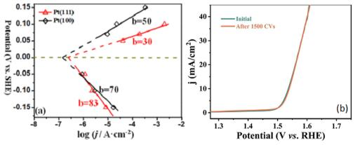
Fig. 3 (a) Typical Tafel plots showing oxidation and reduction half reactions for single crystal Pt, reprinted with permission from the American Chemical Society, Fang and Liu<sup>73</sup> (b) linear polarisation curves highlighting the stability of CoFe-LDH wrapped on Ni-doped carbon nanorods, reprinted with permission from Elsevier, Zhang and Hao.<sup>75</sup>
