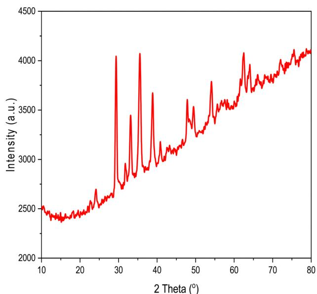
Fig. 2 XRD patterns of copper ferrite (CF).
