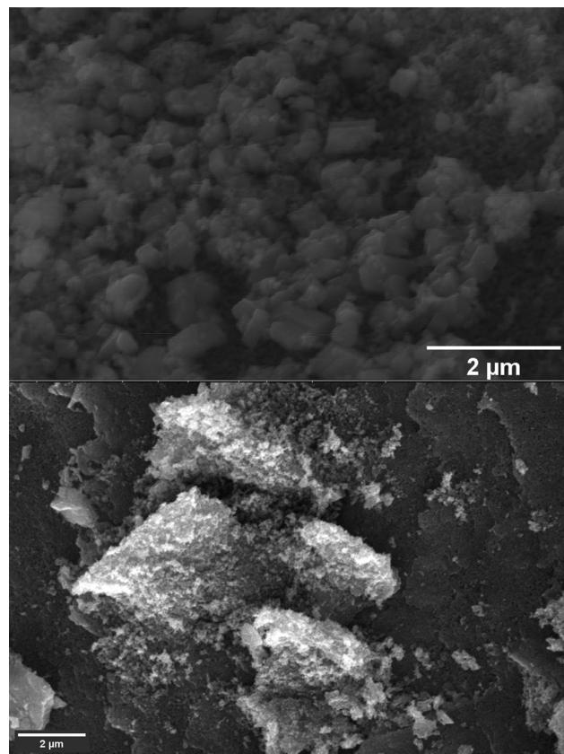
Fig. 4 SEM images of copper ferrite (CF).
