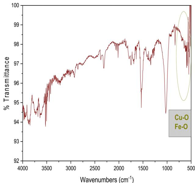
Fig. 1 FTIR spectrum of copper ferrite (CF).
