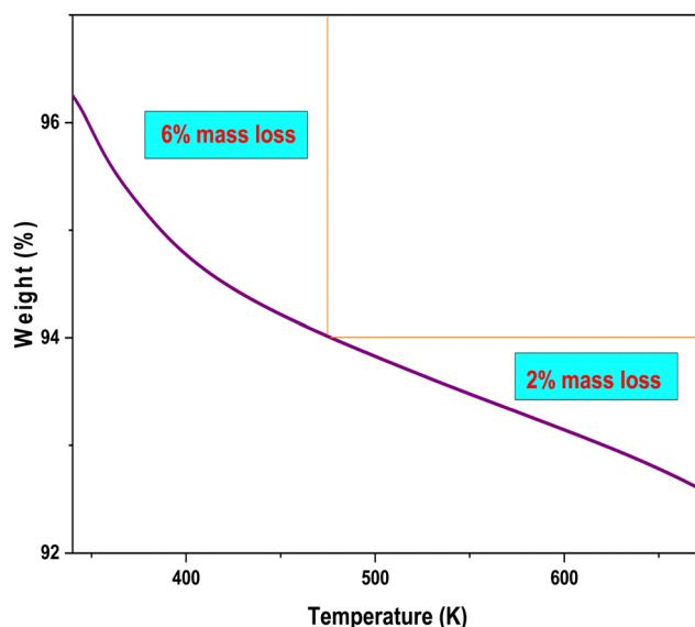
Fig. 3 TG curve of copper ferrite (CF).
