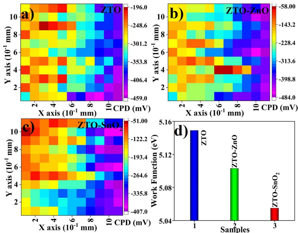
Fig. 4 Contact potential difference of (a) ZTO, (b) ZTO–ZnO, and (c) ZTO–SnO<sub>2</sub> samples coated over the FTO substrates scanned over an area of 1 × 1 mm<sup>2</sup>. (d) The average surface work function of the ZTO, composite ZTO–ZnO, and ZTO–SnO<sub>2</sub> heterostructure samples.
