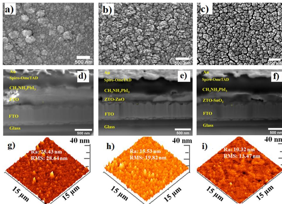
Fig. 2 (a)–(c) FESEM surface morphology images of fabricated ZTO, ZTO–ZnO, and ZTO–SnO<sub>2</sub> ETL-based perovskite solar cell devices, respectively. (d)–(f) FIB cross-sectional images of the ZTO, ZTO–ZnO, and ZTO–SnO<sub>2</sub> ETLs used in PSC devices. (g)–(i) AFM images of ZTO, ZTO–ZnO, and ZTO–SnO<sub>2</sub> coated on FTO substrates, respectively.
