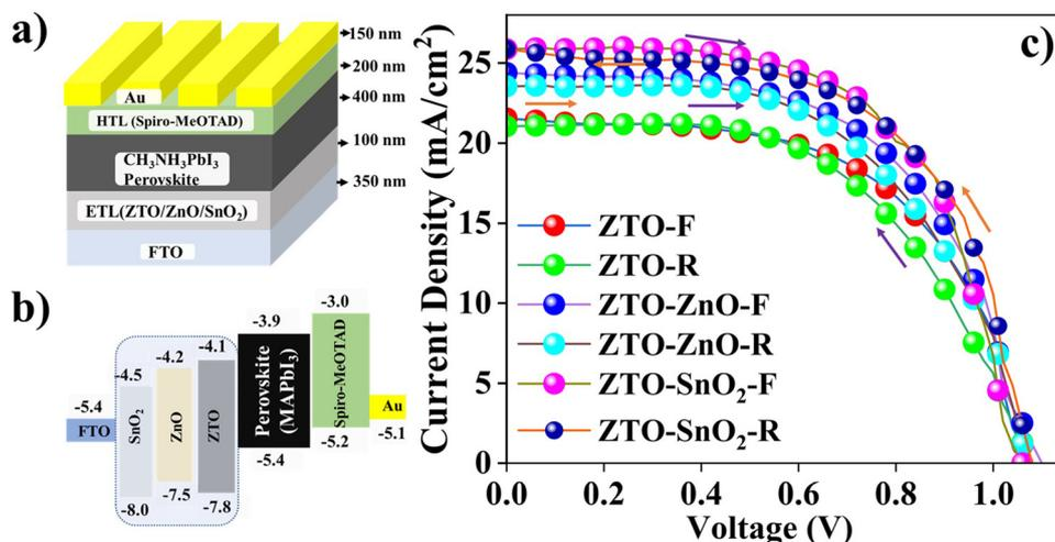
Fig. 6 (a) Schematic representation of the fabricated ZTO/ZTO-ZnO/ZTO-SnO<sub>2</sub> electron transport layers used in PSC devices with appropriate film thicknesses, (b) energy band diagram of the different ETL-based PSC device, and (c) *J-V* curves of the fabricated PSC device results compared with forward and reverse bias conditions.
