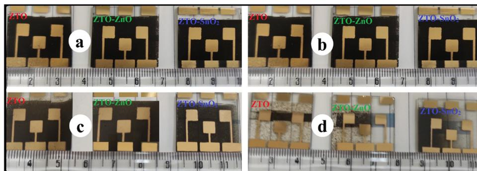
Fig. 10 Visible degradation of the pristine ZTO, and composite ZTO-ZnO, ZTO-SnO<sub>2</sub> heterostructure-based PSC devices; (a) as-fabricated, (b) after 10 days, (c) after 20 days, and (d) after 30 days.
