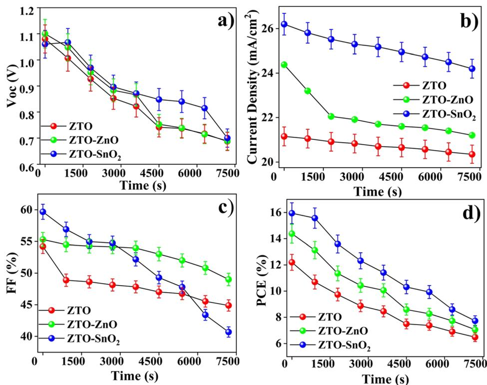
Fig. 9 (a) Stability egging test for the pristine ZTO, and composite ZTO-ZnO, ZTO-SnO<sub>2</sub> heterostructure-based PSC devices; open-circuit voltage, (b) short circuit current, (c) fill factor, and (d) power conversion efficiency.
