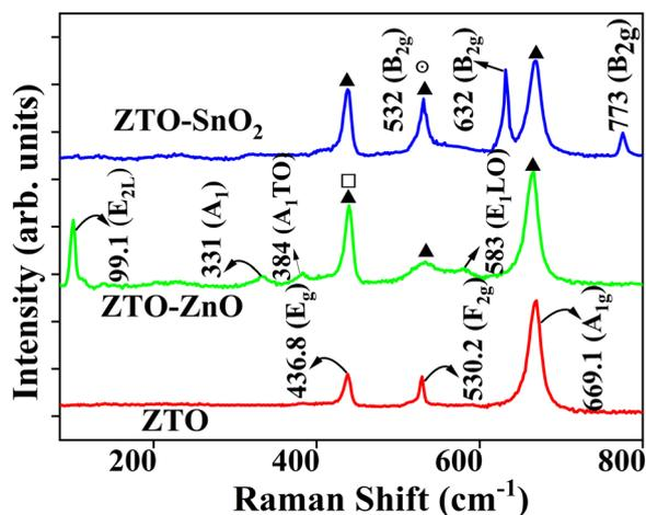
Fig. 5 Raman spectra of synthesized ZTO, ZTO-ZnO, and ZTO-SnO<sub>2</sub> heterostructure samples.
