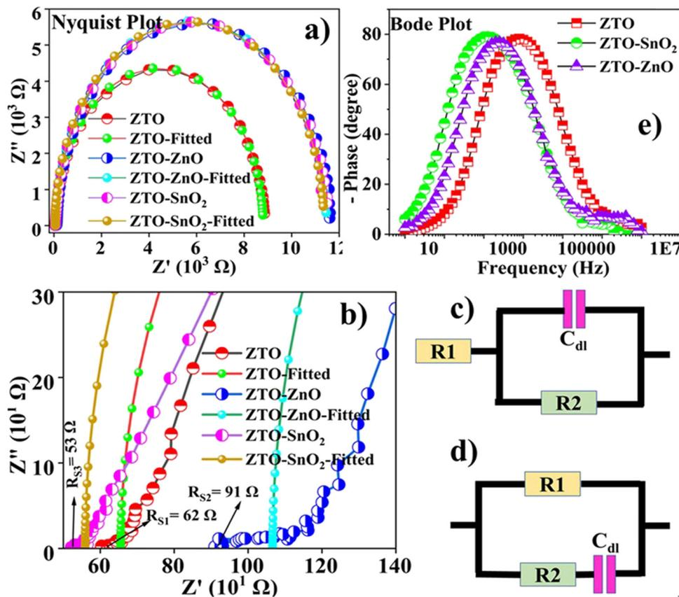
Fig. 8 (a) Electrochemical impedance spectra (Nyquist plot) of ZTO, ZTO–ZnO, and ZTO–SnO<sub>2</sub> ETL-based PSC devices, (b) extended view of the Nyquist plot in the higher frequency range, (c) and (d) the equivalent circuit used for the  $J$ – $V$  curve analysis, and (e) Bode plot of the fabricated devices.
