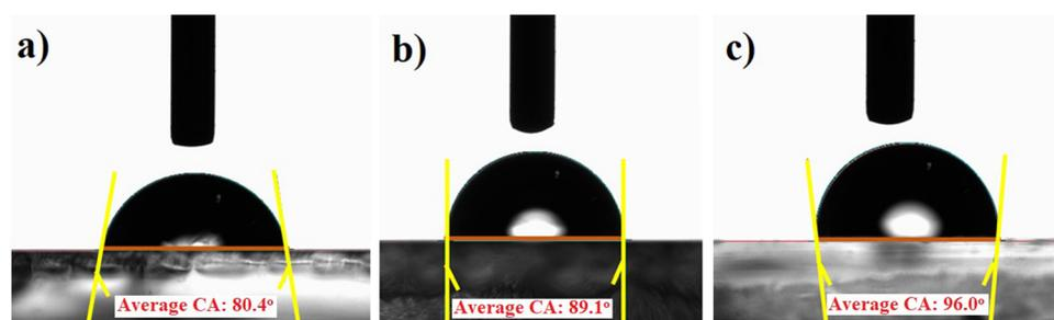
Fig. 3 Contact angle measurement of the synthesized (a) pristine ZTO, (b) ZTO–ZnO, and (c) ZTO–SnO<sub>2</sub> samples coated over FTO substrates.
