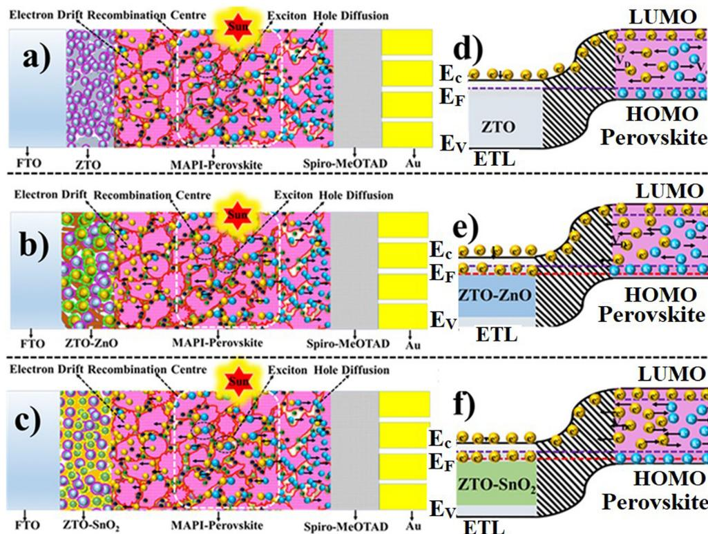
Fig. 7 Schematic representation of pristine ZTO (a) and (b), ZTO–ZnO (c) and (d), and ZTO–SnO<sub>2</sub> (e) and (f) heterostructure-based ETLs used in PSC device structures and with an appropriate energy band diagram with different ETLs.
