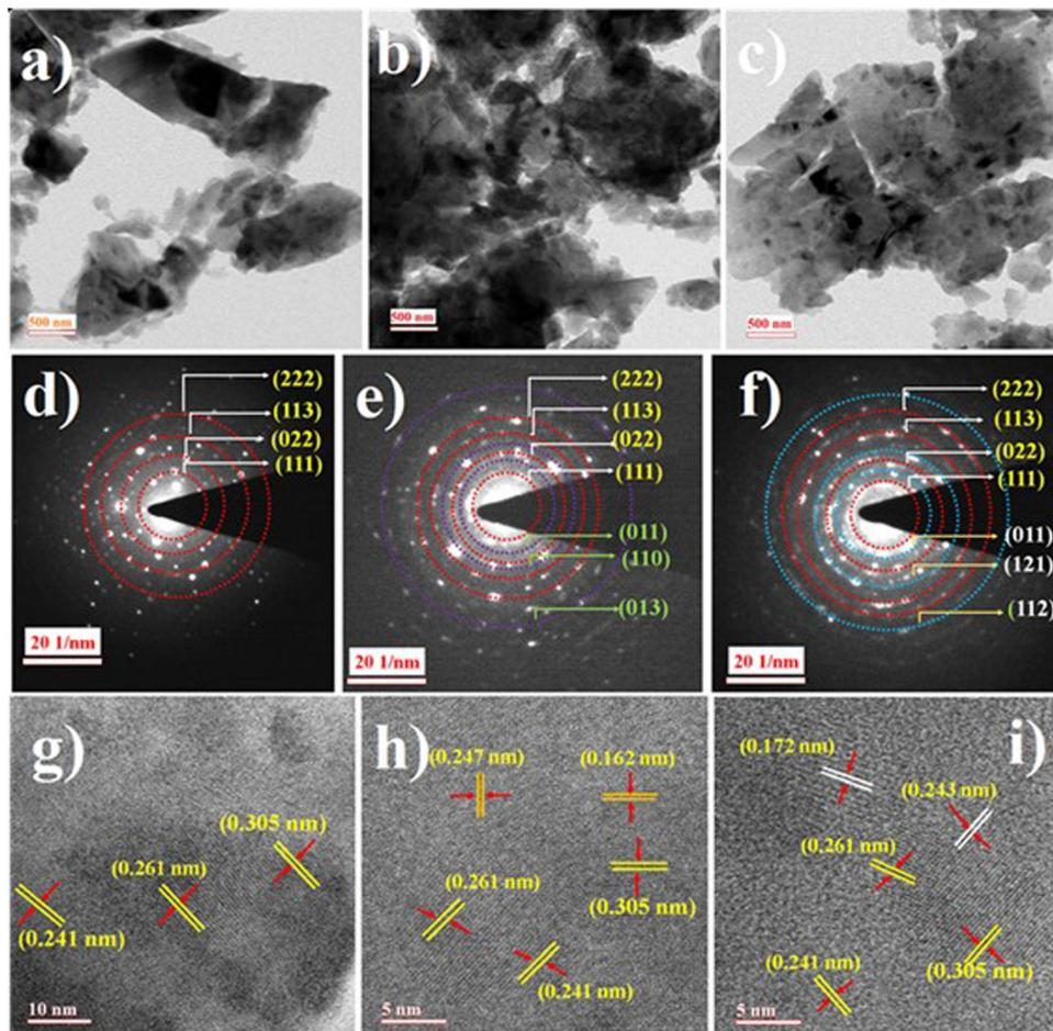
Fig. 1 Synthesized ZTO, ZTO-ZnO, and ZTO-SnO<sub>2</sub> samples topological features from the TEM (a)–(c), SAED (d)–(f), and HR-TEM (g)–(i) images indicating the heterostructure formation.
