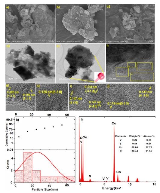
Fig. 3 (a)–(c) SEM images of the CoO<sub>x</sub>–S–VO<sub>x</sub> material, (d)–(f) TEM images, (g)–(j) are enlarged images marked as 1–4 in f, (k) particle size distribution curve, (I) the EDX spectra showing the elemental distribution in the catalyst.
