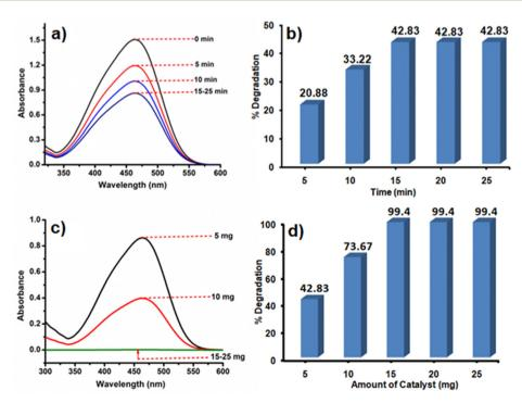
Fig. 6 UV spectra and bar diagram showing the dependence of MO degradation on time (a) and (b), and catalyst amount (c) and (d).
