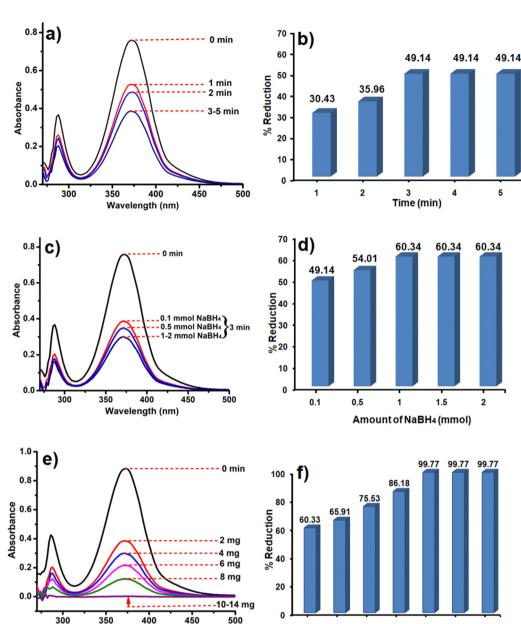
Fig. 5 UV spectra and bar diagram showing the dependency of Cr(vi) reduction on time (a) and (b), NaBH<sub>4</sub>concentration (c) and (d) and catalyst amount (e) and (f).
