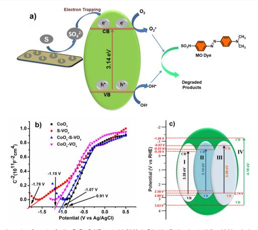
Fig. 8 (a) Plausible charge transfer routes for the CoO<sub>x</sub>-S-VO<sub>x</sub> material, (b) Mott-Schottky (flat band potential) and (c) band edge structure plot of all the catalysts, (I)  $COO_x$  (II)  $COO_x$ -S- $VO_x$ , (III)  $CO_3O_4$ - $V_2O_5$ , (IV) S- $VO_x$ . [Flat band potential ( $E_{FB}$ ) = Conduction band potential ( $E_{CB}$ ) + 0.1 V, Valance band potential ( $E_{VB}$ ) = Band gap +  $E_{CB}$ ].<sup>83</sup>
