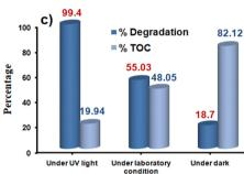
Reaction conditions Fig. 7 (a) UV spectra recorded over a 5 min time interval under optimized reaction conditions, (b)  $\ln(C_n/C_t)$  vs. time graph depicting a kinetic mechanism for MO degradation, and (c) comparative bar diagram of TOC and percentage degradation under various conditions.
