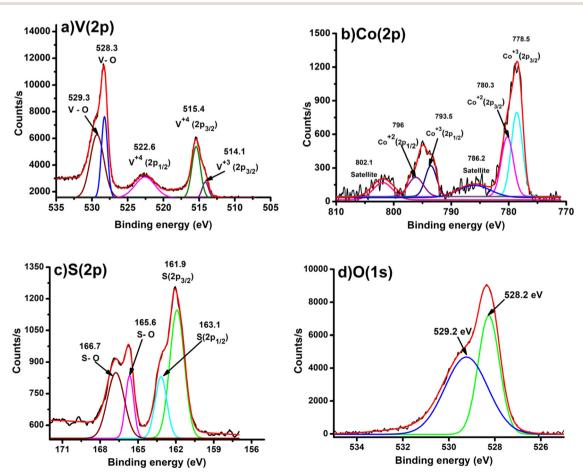
Fig. 2 XPS spectra of (a) V(2p), (b) Co(2p), (c) S(2p), and (d) O(1s) present in  $CoO_x$ -S-VO<sub>x</sub>.
