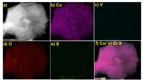
Fig. 4 (a) Region selected for STEM-HAADF-EDX mapping of the  $CoO_x$ -S-VO $_x$ material showing the presence of all the elements, (b) Co, (c) V, (d) O, (e) S, (f) mixing of all elements.
