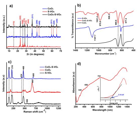
Fig. 1 (a) XRD pattern of CoO<sub>x</sub> (blue), S-VO<sub>x</sub> (red) and CoO<sub>x</sub>-S-VO<sub>x</sub>(black). (b) FTIR spectra of CoO<sub>x</sub> (black), S-VO<sub>x</sub> (blue) and CoO<sub>x</sub>-S-VO<sub>x</sub> (red). (c) Raman spectra of CoO<sub>x</sub> (red), S-VO<sub>x</sub> (black) and CoO<sub>x</sub>-S-VO<sub>x</sub> (blue) and (d) DRS spectra of CoO<sub>x</sub>-S-VO<sub>x</sub>, with the inset showing Tauc plot.
