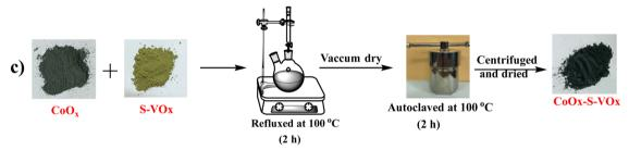
**Scheme 1** Schematic representation of the preparation of the  $CoO_x$ -S-VO<sub>x</sub> catalyst.
