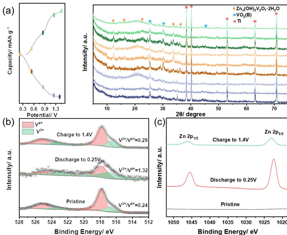
Fig. 5 *Ex situ* structural characterizations of VO<sub>2</sub>@C-350 electrode in the 1st cycle. (a) XRD patterns, (b) V 2p XPS spectra, and (c) Zn 2p XPS spectra.
