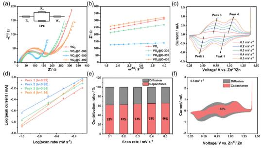
Fig. 4 (a) Nyquist plots and equivalent circuit of VO<sub>2</sub>-based samples. (b) Correlation between Z' and  $\omega^{-1/2}$ . (c) CV curves for VO<sub>2</sub>@C-350 at 0.1–0.5 mV s<sup>-1</sup>. (d) Log(i) versus log(v) plots of VO<sub>2</sub>@C-350. (e) Contribution of capacitive ion storage of VO<sub>2</sub>@C-350 at 0.1–0.5 mV s<sup>-1</sup>. (f) Contribution of capacitive ion storage of VO<sub>2</sub>@C-350 at 0.5 mV s<sup>-1</sup>.
